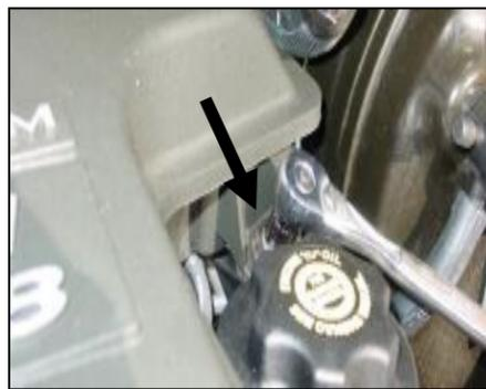
**2.** Loosen the two 10mm bolts securing the factory resonator to the intake manifold.
