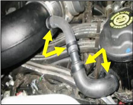
**17. 2003 Models Only:** Use the plastic barbed fitting and 1/2" hose provided; connect factory vent hose to Airaid intake tube & secure the 1/2" hose with (2) #16 black speed clamps provided. Secure factory vent hose with (2) #22 black speed clamps provided.
