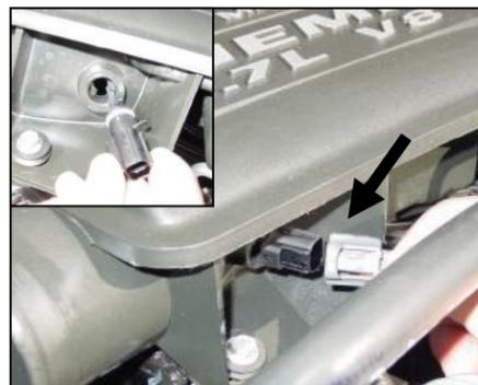
**3.** Disconnect the air temperature sensor connector on the front of the factory resonator. Next, twist the temperature sensor and remove it from the factory intake resonator. (Retain for later use with Airaid intake).
