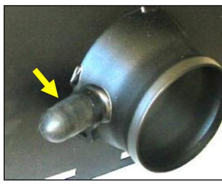
**10. 2003 Models Only:** Slip the black rubber cap over the nipple on the Cool Air Dam and secure using the #19 black speed clamp provided.
