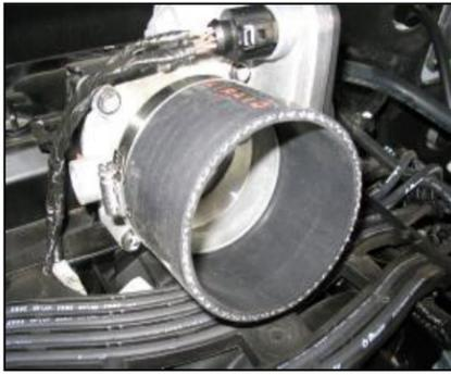
**14.** Slide the urethane coupler onto the throttle body and secure using a #60 hose clamp provided & install the 2nd #60 hose clamp on the other end of the coupler, leave loose for final assembly.
