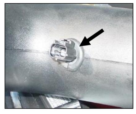
**12.** Install the rubber grommet into the hole on the back side of the Airaid tube & insert the factory air temp sensor into grommet.
