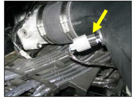
**16.** Re-connect air temperature sensor connector.
