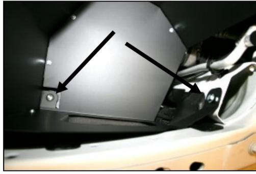
**11.** Install the CAD assembly into the vehicle, and install the 3/8-16x1 1/4" button head bolt (#18) thru the panel, and into the well nut. Next install the 6x1x12mm hex bolt (#16), and 1/4" flat washer (#12), thru the panel, and into the captured nut in the radiator support. Leave all bolts loose until final adjustment.
