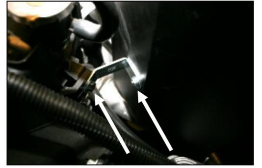
**12.** Using one 1/4-20x1/2" button head bolt (#11), 1/4" flat washer (#12), and 1/4" serrated nut (#13), and the 8x1.25x30mm hex bolt (#14), and 5/16" flat washer (#15), mount the supplied bracket (#19) between the CAD panel, and the fan shroud mounting boss as shown. Tighten all CAD mounting bolts at this time.
