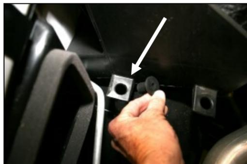
**8.** Install the supplied well nut (#21) into the support bracket hole that is closest to the fender.
