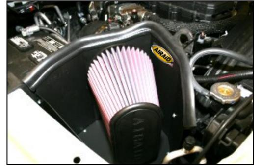
**15.** Install the Airaid Premium Filter (#1) onto the Airaid filter adapter, and tighten the hose clamp. Install the weather strip (#7) onto the top of the CAD, starting at the fender, and working your way towards the radiator.
