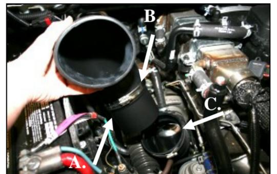
**9.** **A)** Install the metal tube (#5) into the rubber elbow (#6) until the rolled bead touches the side. **B)** Install one #80 hose clamp (#20) around the elbow at the metal tube, and tighten. **C)** Install the tube assembly into the factory rubber elbow on the turbocharger. Leave the factory hose clamp loose until final adjustments are made.
