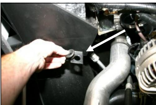
**7.** Remove the two factory rubber grommets that held the factory airbox base in place.
