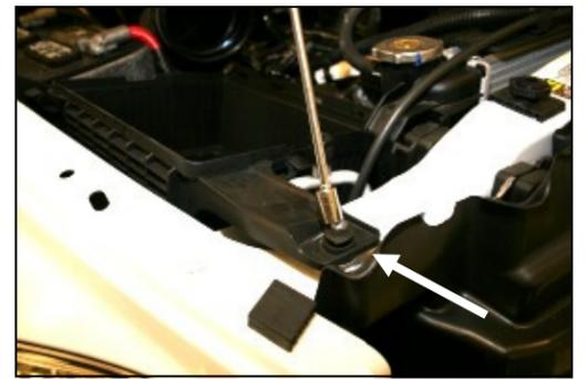
**3.** Using a 10mm socket, remove the nut that holds the front of the airbox base and grommet assembly to the radiator support.
