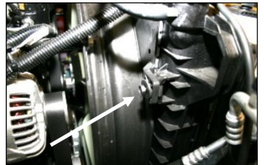
**6.** Using a 13mm socket, remove the factory bolt that holds the fan shroud to the radiator.
