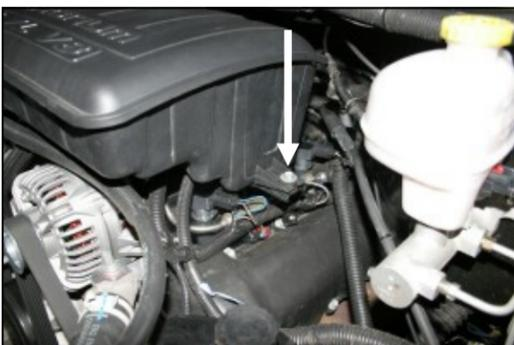
**4.** Using a 10mm socket, remove the two bolts (one bolt on 2008 and newer models) that secure the intake resonator to the engine, one on the drivers side, and one on the passenger side of the resonator. Grab the resonator with both hands at the front and push back and up to release it from the locator grommet on the bottom. Remove the resonator from the vehicle.
