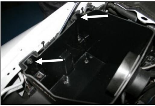
10. Install the CAB into the vehicle aligning the grommets over the locating pins. Reinstall the two factory bolts into the fender that were removed in step #9.
