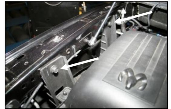
**3.** Using a 13mm socket, remove the two bolts that hold the air cleaner mount to the inside right fender. Save them for reinstallation in step #10.
