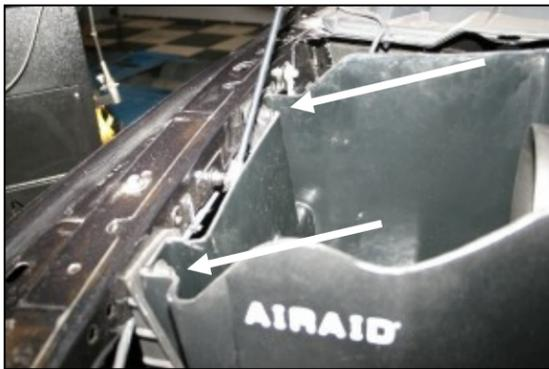
**10.** Install the CAB into the vehicle by aligning the grommets over the locating pins on the factory airbox mount. Reinstall the factory bolts into the fender that were removed in step #3.
