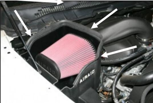
**17.** Install the Airaid Premium Filter (#1) onto the filter adapter and tighten the clamp. Next install the weather strip (#8) on the top of the CAB as shown. (Hint: Start at one end of the CAB and work your way towards the other end.)
