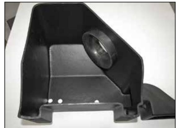
7. Install the filter adapter into the air box as shown and secure with the provided hardware.
