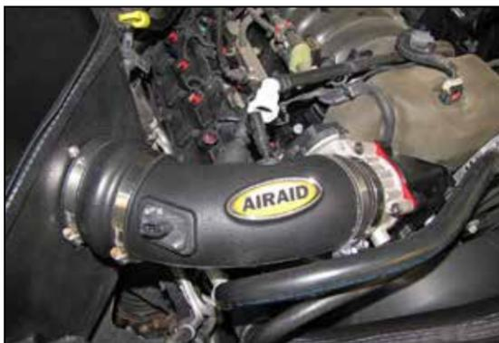
15. Install the AIRAID® intake tube into the hump coupler and onto the throttle body, adjust the tube and couplers for best fit and then secure with the provided hose clamps.
