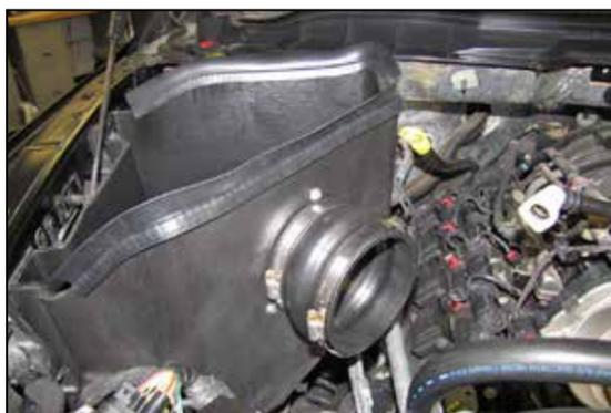
14. Install the provided hump coupler onto the filter adapter as shown.
