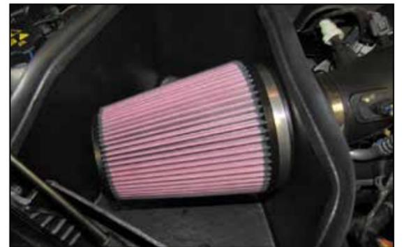
17. Install the air filter onto the filter adapter and secure with the provided hardware.
