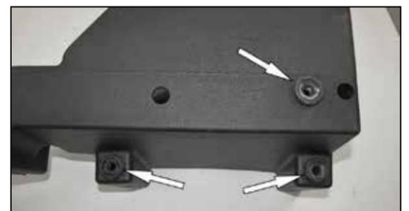
8. Remove three of the factory mounting grommets from the factory air filter housing and install them as shown into the AIRAID® air filter housing.
