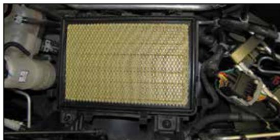
5. Lift the lower air filter housing up and then remove the housing from the vehicle.
