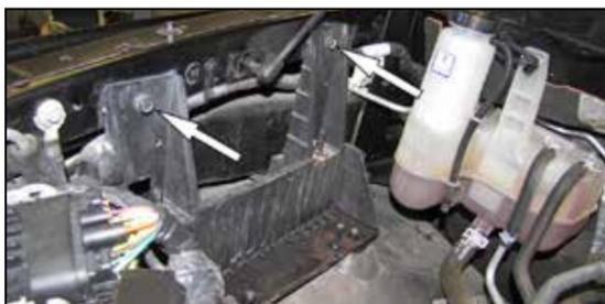
6. Remove the two upper filter housing bracket mounting bolts.
