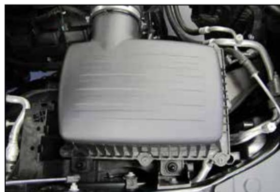
4. Pull up the factory air filter assembly to dislodge it from the mounting posts and then remove the complete intake assembly from the vehicle.
