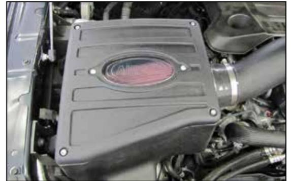
16. Install the AIRAID® window into the air filter housing lid and then install the lid onto the air filter housing and secure with the provided hardware.
