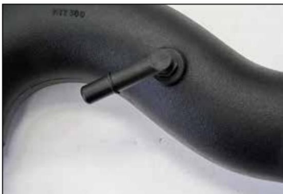
9. Install the provided quick disconnect fitting into the AIRAID® intake tube as shown.
