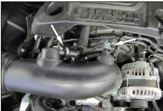
2. Disconnect the inlet air temperature sensor electrical connection and crank case vent quick disconnect fitting.
