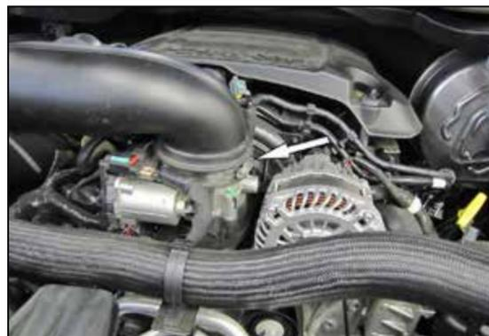
3. Loosen the hose clamp that secures the factory intake tube to the throttle body.
