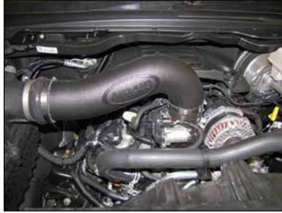
10. Install the AIRAID® intake tube into the coupler at the air filter housing and then into the coupler at the throttle body, adjust the tube for best fit and then secure with the provided hose clamps.
