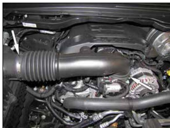
3. Loosen the hose clamps that secure the factory intake tube and then remove the intake tube from the vehicle. **NOTE:** AIRAID recommends that customers do not discard factory air intake.
