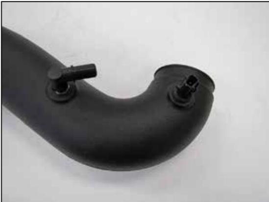
9. Install the Grommet supplied into the AIRAID® intake tube and then install the inlet air temperature sensor into the grommet. Install the provided vent fitting into the AIRAID intake tube as shown.
