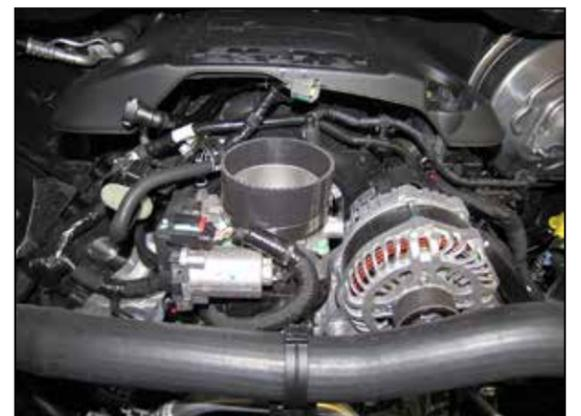
6. Install the coupling hose (KITCOUPLER09) onto the throttle body and secure with the provided hose clamp.
