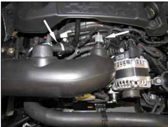
2. Disconnect the crank case vent line from the factory intake tube and disconnect the inlet air temperature sensor electrical connection.
