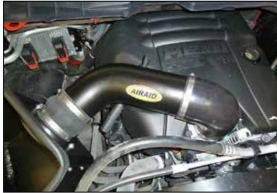
25. Install the AIRAID intake tube into the silicone hump hose and then into the silicone hose at the throttle body. Align the heat shield assembly for proper fit and then tighten the heat shield mounting bolts then tighten the hose clamps securing the intake tube.
