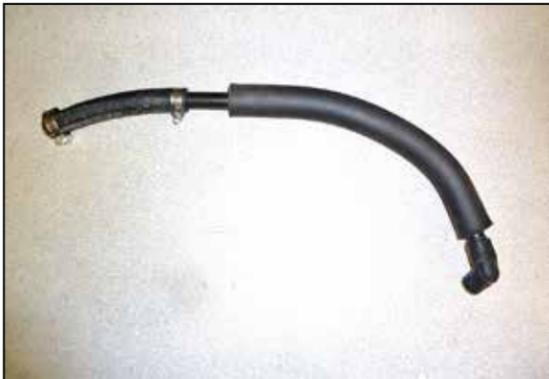
9. Install the provided silicone crank case vent hose onto the cut end of the factory crank case vent tube as shown.
