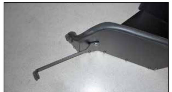
17. Install the heat shield mounting bracket (083103-1A) onto the heat shield using the provided hardware.
