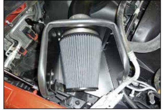
28. Install the AIRAID air filter and secure with the provided hose clamp.
