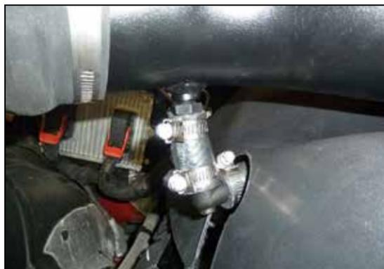
26. Connect the crank case vent hose to the vent fitting installed into the AIRAID intake tube. Secure with the provided tie wrap.
