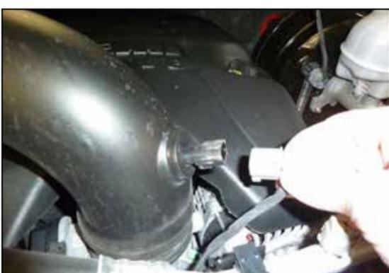
2. Release the red locking tab and then disconnect the inlet air temperature electrical connection.
