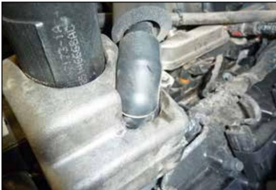
10. Install the crank case vent assembly onto the valve cover port.
