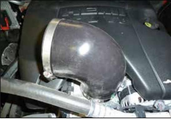
21. Install the provided 90° silicone hose onto the throttle body and secure with the provided hose clamp.
