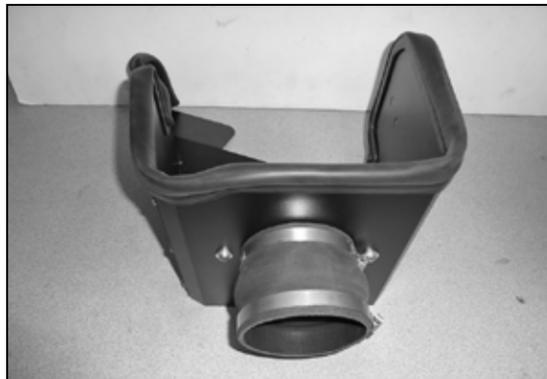
15. Install the silicone hump hose onto the filter adapter and secure with the provided hose clamp.
