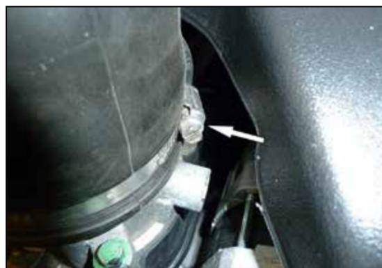
3. Loosen the hose clamp which secures the intake tube to the throttle body.
