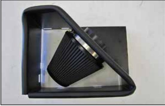
9. Install the AIRAID® air filter onto the filter adapter and secure with the provided hose clamp.
