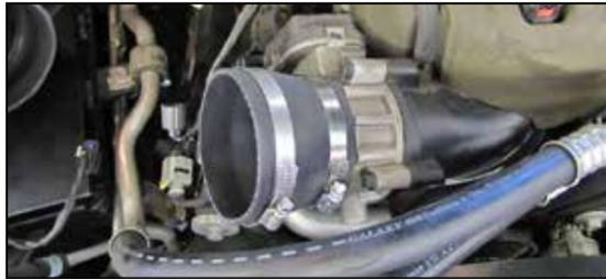
16. Install the provided step coupler (08497) onto the throttle body and secure with the provided hose clamps.
