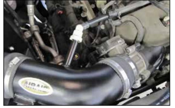
18. Connect the factory crankcase vent hose to the quick disconnect fitting on the AIRAID® intake tube.
