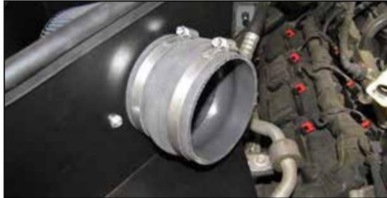
15. Install the provided coupler hump hose (08418) onto filter adapter and secure with the provided hose clamp.
