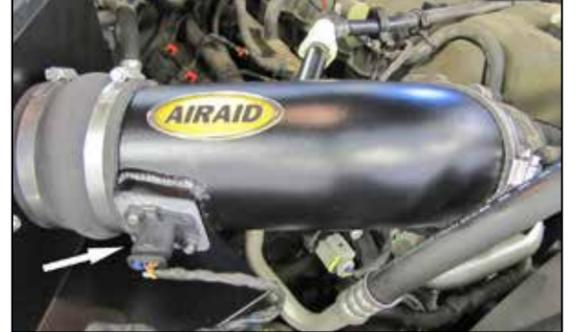
19. Reconnect the humidity sensor and inlet air temperature sensor electrical connections.
