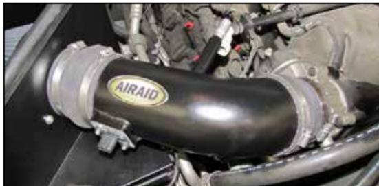
17. Install the intake tube into the hump coupler and then into the step coupler, then adjust the tube for best fit and secure with the provided hose clamps.
