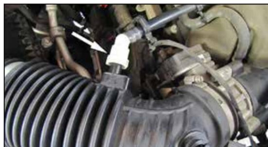
4. Depress the locking tab and then disconnect the crank case vent hose from the factory intake tube.
