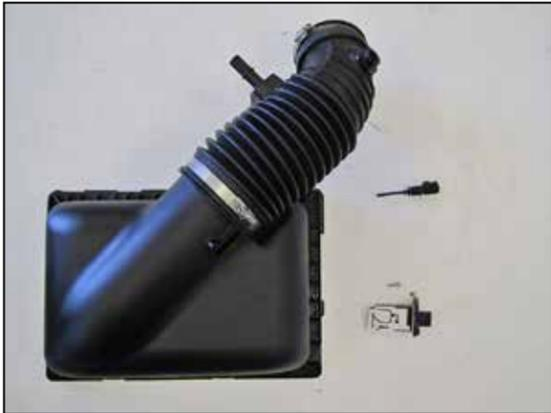
11. Remove the two screws securing the mass air sensor then remove the sensor from the air filter housing. Remove the inlet air temperature sensor from the stock intake tube.
