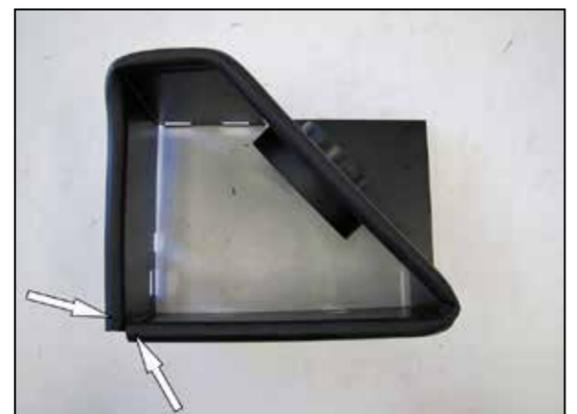
8. Install the provided edge trim onto the heat shield as shown.
