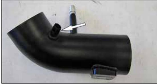
13. Remove the O-ring from the inlet air temperature sensor and then install the sensor into the grommet installed into the intake tube during the previous step.
