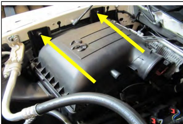
4. Remove the two fender bolts in the air box cradle and remove the entire air box assembly. The bolts will be reused in step 10.
