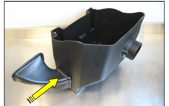
6. Transfer the air scoop from the factory airbox into the Airaid cool air box as shown.
