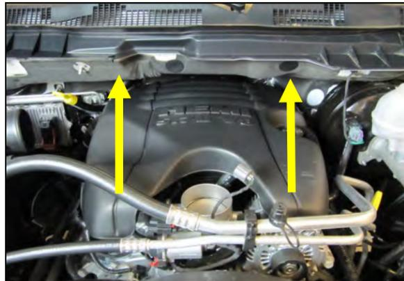
2. Lift the front of the engine cover up to unseat it from the mounting grommets and remove it.
