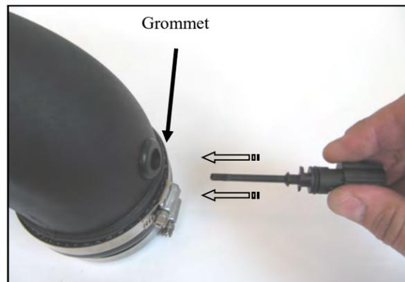
15. Insert the 1/2" grommet into the Airaid Intake tube. Transfer the air temperature sensor from the factory intake tube, into the Airaid Tube. Hint: A small amount of silicone or soapy water makes for a safe grommet/o-ring lubricant.
