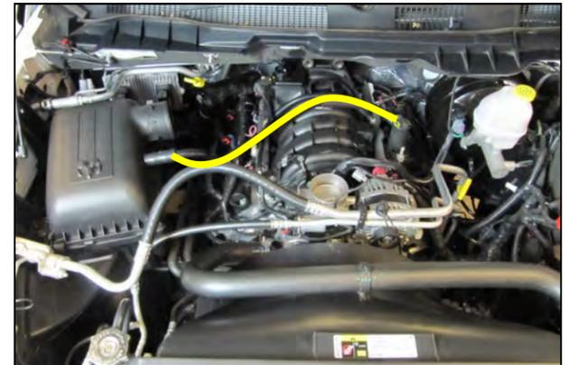
2. Remove the PCV line connecting the air box to the valve cover. Note: The 90 degree fitting on the valve cover is to remain in place.
