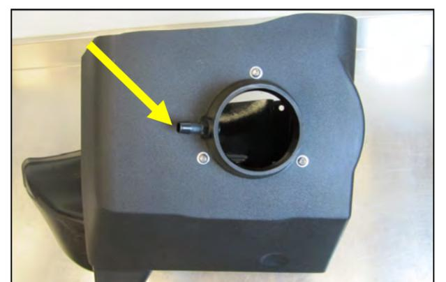
9. Install the 1/4" barbed fitting into the cool air box snout as shown.
