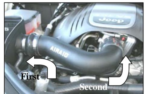
18. Carefully install the end of the Airaid Intake Tube (#4) into the hump hose, and then into the reducer on the throttle body as shown. Adjust the tube as needed, and then **tighten the four hose clamps**.
