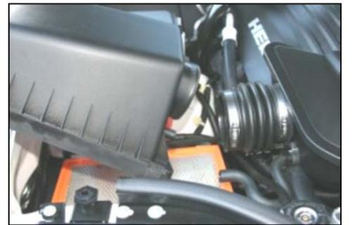
3. Remove the air cleaner box lid by sliding it forward, and then up, and out of the factory intake tube.
