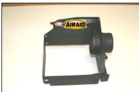
11. Assemble the two pieces of the Quick Fit panels as shown (#2&#3), using the four 6-32 screws (#12), washers (#13), and nuts (#14), that are provided in the kit. Apply the Airaid Foil Decal onto the Panel as shown.
