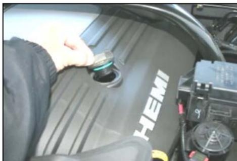
5. Remove, and set aside the oil filler cap.
