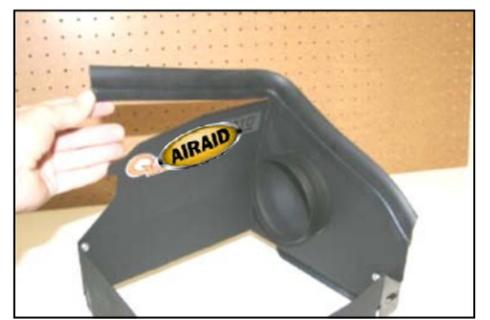
12. Install the weather strip (#7) on the top of the Quick Fit assembly. (*Hint: start at one end, and go towards the other end, don't start in the middle.*)
