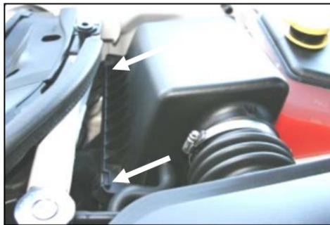
2. Unhook the two air cleaner lid latches on the front of the airbox.
