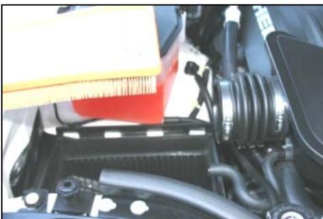
4. Remove factory air filter from the air cleaner box.
