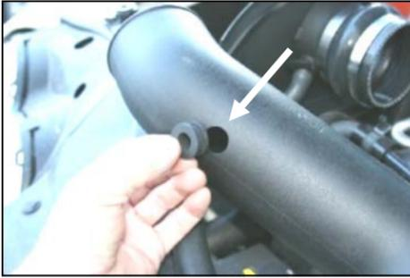
16. Install the supplied grommet (#8) into the hole in the back of the tube.
