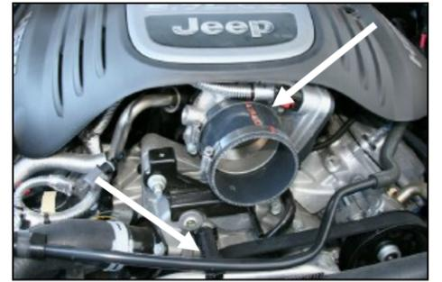
15. Install the reducer (#6) and two #56 hose clamps (#9) on the throttle body as shown. **Do not tighten** the clamps at this time. Secure the breather hose to the air conditioner line using the supplied zip tie (#15).
