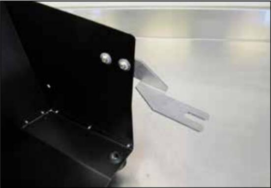
11. Install the Mounting Bracket (#6) onto the Panel assembly using the two 1/4-20 Button Head Bolts (#8), 1/4" Flat Washers (#9), and 1/4-20 Flange nuts (#10).
