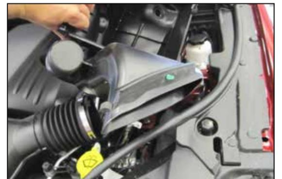
6. Unseat the lower half of the factory airbox from its mounting grommets and remove the airbox and air inlet duct as an assembly.
