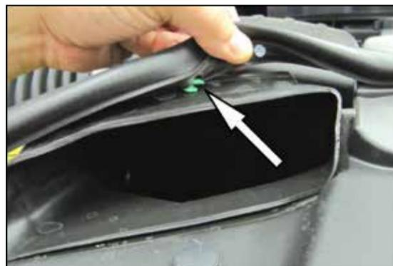
5. Carefully separate the hood seal from the cleat on the airbox inlet. Pull gently from side to side to avoid tearing the seal.
