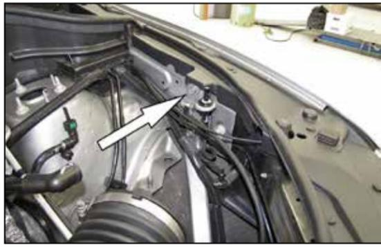
12b. On vehicles that are equipped with electronic power steering, remove the bolt shown from the inner fender and set aside. This bolt will be reused in a later step to hold the Mounting bracket.
