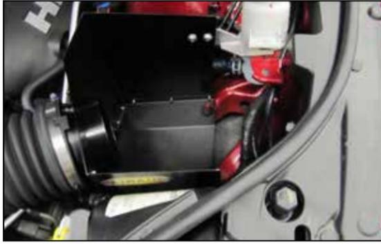
13. Install the Panel assembly into the engine compartment as shown. On vehicles equipped with a power steering reservoir, slide the Mounting bracket underneath the power steering reservoir and the airbox mounting post through the grommet in the Panel. Secure the assembly by reusing the bolt from step 12a. On vehicles that are equipped with electronic power steering, secure the assembly using the bolt from step 12b. Connect the factory intake tube to the Airaid Intake tube and tighten the clamp.
