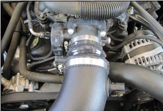
13. Open and Install the Clamps onto the Coupler as shown with the #44 clamp on the throttle body (#9) and the #52 clamp (#8) on the Intake Tube.
