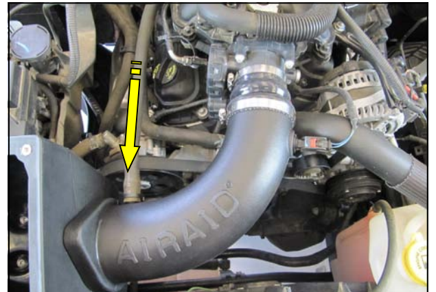
15. Reconnect the factory crank case breather line to the Airaid Intake Tube.
