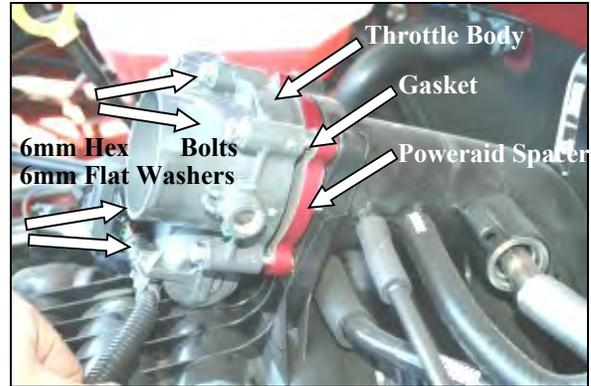
4. Install the Airaid Spacer (#1) with the bore extending into the intake manifold. Install the Gasket (#2) between the Airaid Spacer and the throttle body. Install four 6mm x 50mm hex bolts (#3) and 6mm flat washers (#4) through the throttle body, AiraidSpacer, Gasket, and into the intake manifold. Using a 10mm socket, tighten all four throttle body bolts evenly, to the manufacturer's specifications. **Do Not Over Tighten The Bolts!** Reference picture below for spacer orientation.
