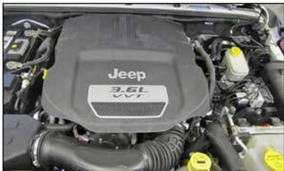
2. Lift up and remove the engine cover.
