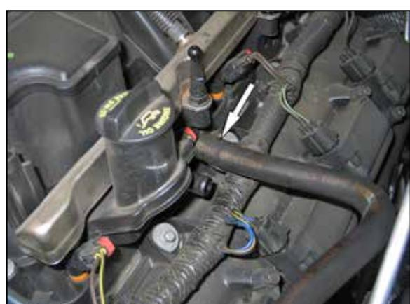
5. Disconnect the crankcase vent hose from the valve cover port.
