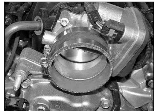
17. Install the provided hose onto the throttle body and secure with the provided hose clamp.
