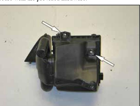
11. Remove two of the factory airbox mounting grommets from the lower airbox.
