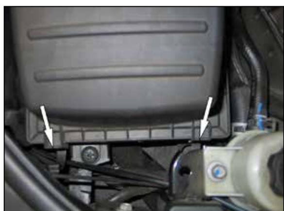
6. Release the two upper airbox retaining clips.
