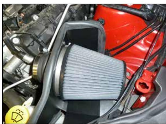
16. Install the AIRAID® filter onto the adapter and secure with the provided hose clamp.
