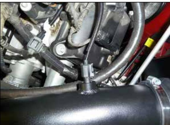
22. Connect the inlet air temperature sensor extension harness into the factory electrical connection and then connect the other end into the inlet air temperature sensor as shown.
