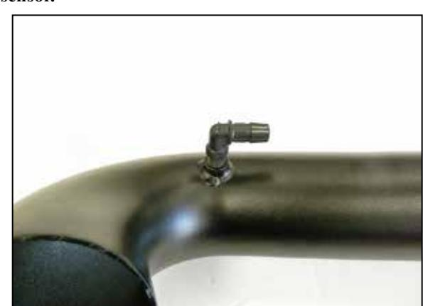
19. Install the 90° npt fitting into the AIRAID® intake tube as shown.
