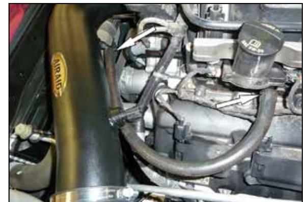
21. Install the crankcase vent hose onto the 90° vent fitting and then attach the open end to the valve cover port.
