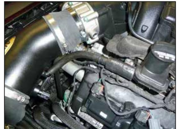
21. Install the assembled vent hose onto the fitting installed in the AIRAID® intake tube and then attach the open end to the valve cover port.
