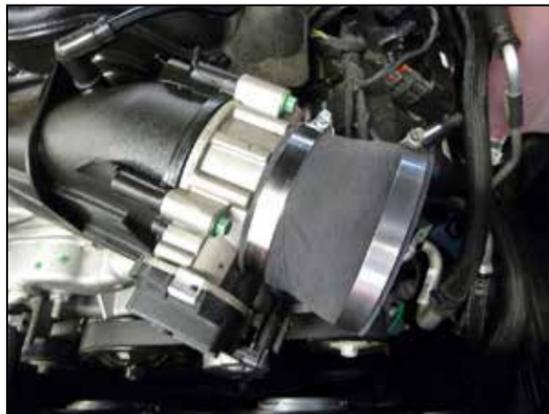
14. Install the step hose (08497) onto the throttle body and secure with the provided hose clamp.
