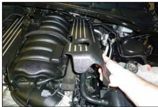
3. Lift up and remove the driver side ignition coil cover as shown.
