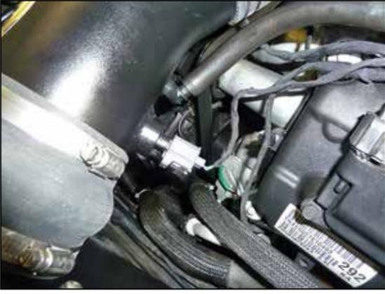
22. Reconnect the inlet air temperature sensor electrical connection.
