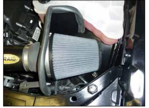
24. Install the AIRAID® air filter and secure with the provided hose clamp.
