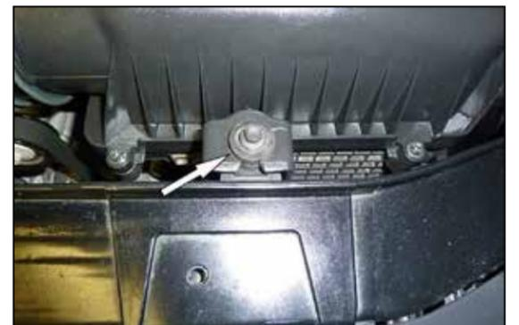
6. Remove the bolt which secures the air box to the core support.
