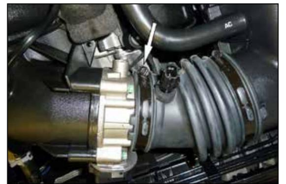
5. Loosen the hose clamp securing the intake tube to the throttle body.
