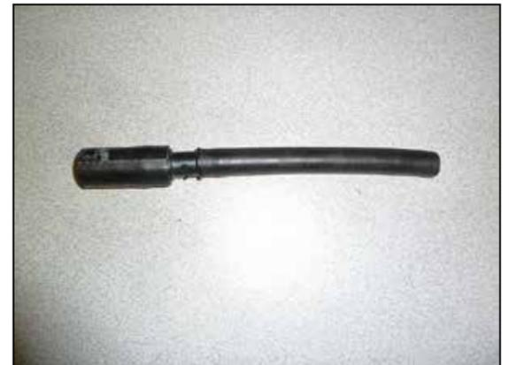
20. Assemble the two vent lines together using the provided hose mender.
