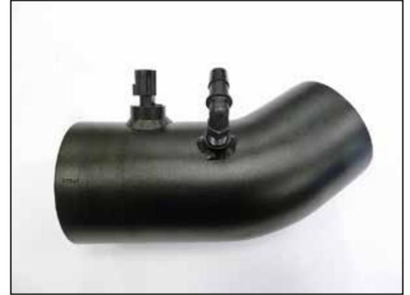
17. Install the inlet air temperature sensor into the AIRAID® intake tube as shown.
