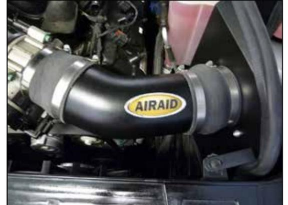
18. Install the AIRAID® intake tube into the silicone hump hose and then into the into the silicone step hose at the throttle body. Align the intake tube and heat shield for proper fit and then secure the intake tube with the provided hose clamps and the heat shield bracket with the factory air box retaining bolt removed in an earlier step.
