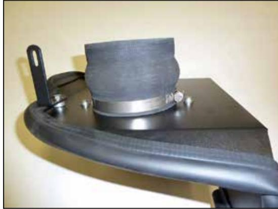
12. Install the provided hump hose (08418) onto the filter adapter and secure with the provided hose clamp.
