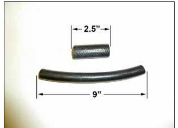
19. Cut the provided 1/2" silicone vent hose to a length of 9" long, and cut the 3/4" vent line to a length of 2.5" long.
