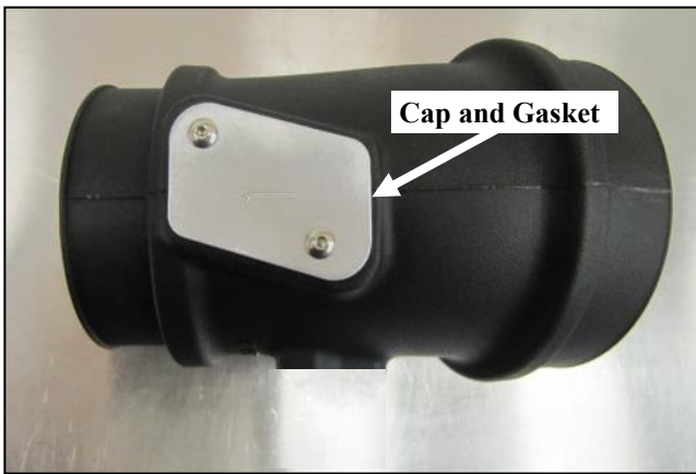
10. Install the Meter Cap and Gasket onto the Airaid Intake tube as shown, using the two 8-32 1/2" Button Head Screws.
