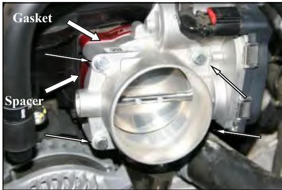
3. Insert the four 6mm x 75mm bolts (#3) with washers (#4) thru the throttle body, one gasket (#2), and thru the Airaid Spacer (#1), and into the intake manifold. Tighten all four throttle body bolts evenly, to the manufacturer's specifications. **Do Not Over Tighten The Bolts!**
