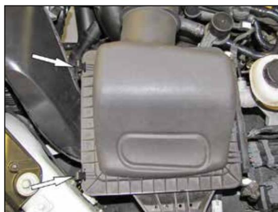
4. Release the two clips that secure the upper air filter housing and then remove the housing and factory air filter.
