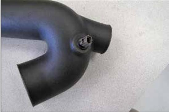
8. Remove the inlet air temperature sensor from the factory intake tube. Remove the O-Ring from the inlet air temperature sensor and then install the sensor into the AIRAID® intake tube using the provided grommet. **NOTE: Use caution while handling the inlet temperature sensor as it is very fragile.**
