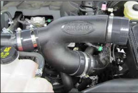
9. Install the AIRAID® intake tube assembly into the coupler and adjust for best fit, then secure the tube with the provided hose clamps.
