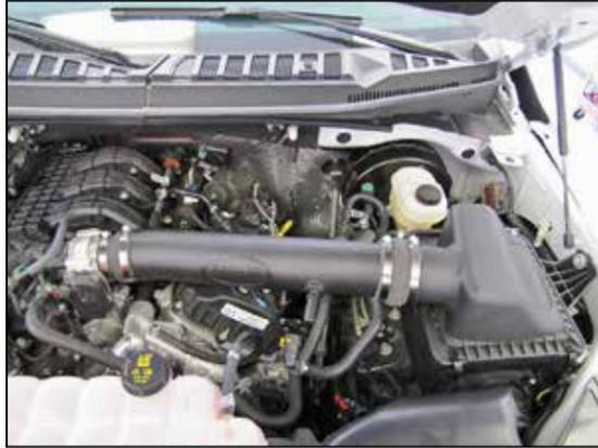
10. Assemble the AIRAID® intake tube and upper air filter housing together loosely, then install the system onto the throttle body and lower housing. Latch the upper air filter housing into position and adjust the intake tube for best fit, then secure with the provided hose clamps.
