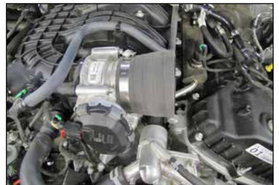
6. Install the provided coupler (084055) onto the throttle body and secure with the provided hose clamp.
