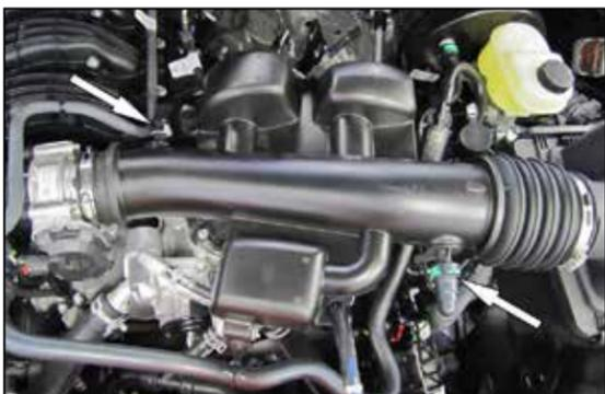
2. Release the locking tabs and then disconnect the crank case vent lines from the intake tube.
