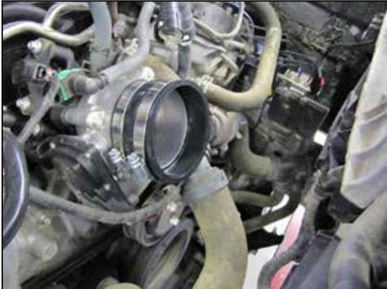
14. Install the provided coupling hose onto the throttle body and secure with the provided hose clamp.
