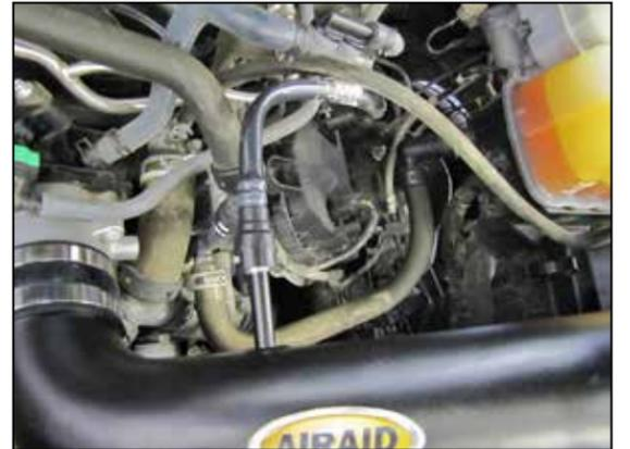
20. Connect the crankcase vent hose to the quick disconnect fitting on the AIRAID® intake tube.
