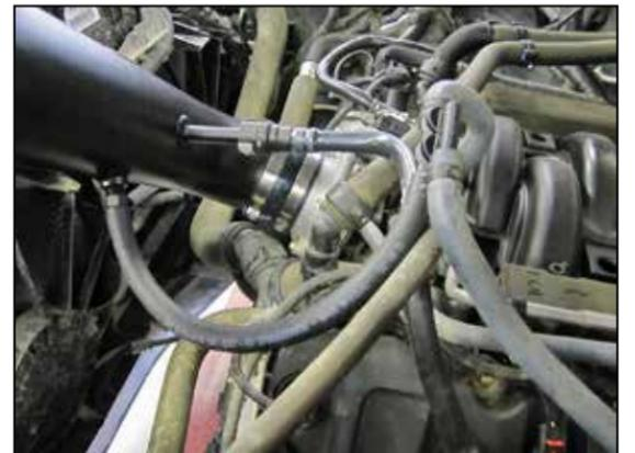
21. Install the provided vent hose onto the 3/8" fitting installed in the AIRAID® intake tube and then attach the open end to the EVAP check valve.
