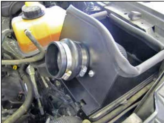
15. Install the provided silicone hose onto the filter adapter and secure with the provided hose clamp.
