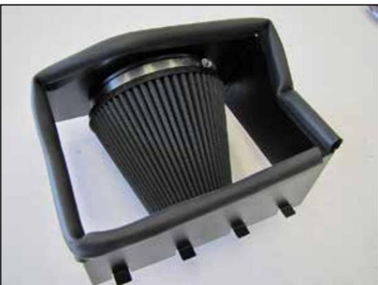
11. Install the AIRAID® air filter onto the filter adapter and secure with the provided hose clamp.
