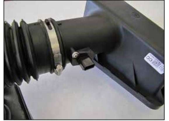
17. Remove the two screws securing the mass air sensor, then remove from the stock intake tube as shown.
