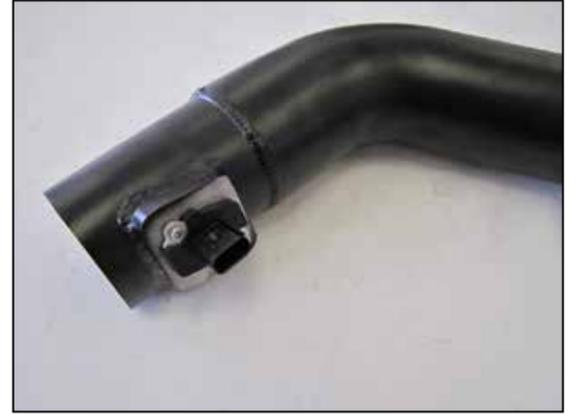
18. Install the mass air sensor into the AIRAID® intake tube and secure with the provided hardware.
