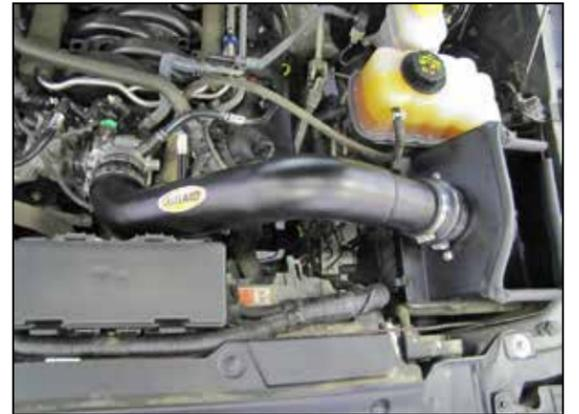
19. Install the AIRAID® intake tube assembly into the hose at the filter adapter and then into the hose on the throttle body and secure with the provided hose clamps.
