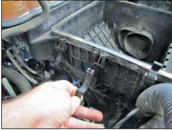
12. Remove the center airbox retaining clip.
