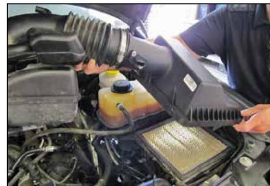
6. Release the three clips securing the upper airbox housing to the lower housing and then remove the intake tube/upper airbox and air filter from the vehicle. **NOTE: AIRAID recommends that customers do not discard factory air intake.**
