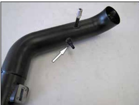
16. Install the provided 3/8" hose fitting into the AIRAID intake tube as shown.
