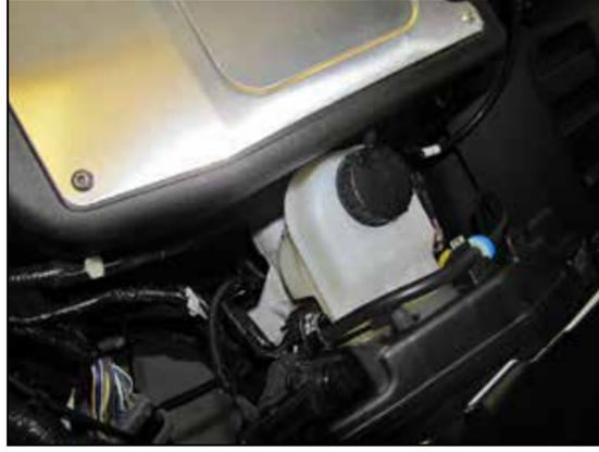
20. Connect the two wiring harness clips to the AIRAID® air filter housing.
