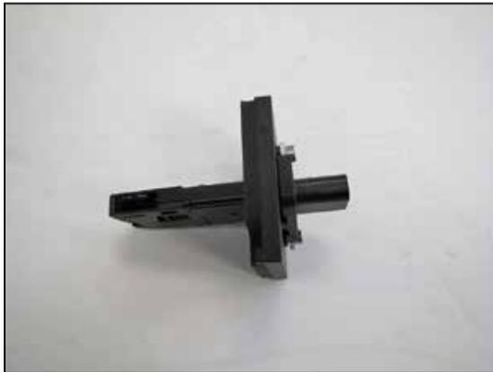
13. Install the provided gasket onto the mass air sensor adapter. Remove the mass air sensor from the factory housing and then install it into the AIRAID® adapter and secure with the provided hardware.
