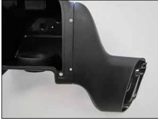
10. Install the AIRAID® fresh air intake duct into the air filter housing and secure with the provided hardware.
