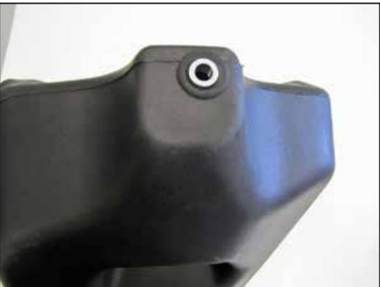
8. Install the provided grommet and spacer into the AIRAID® air filter housing as shown.
