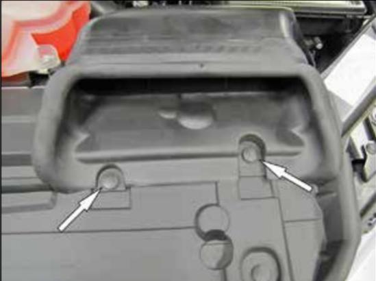
6. Remove the two clips that secure the fresh air intake duct to the core support.
