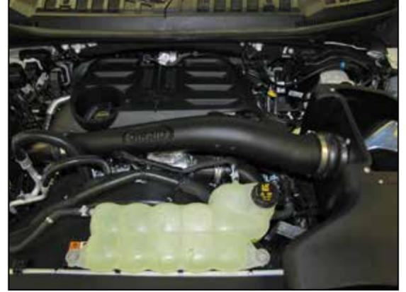
15. Install the AIRAID® intake tube into the factory turbo inlet coupler and the coupler at the filter adapter, adjust the tube for best fit and then secure with the provided hose clamps.
