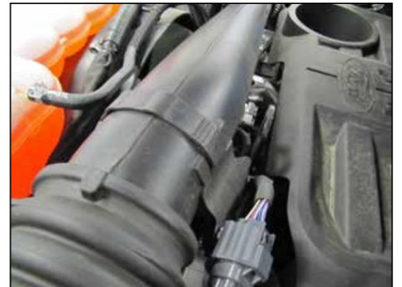
3. Disconnect the mass air wiring harness clip from the intake tube.
