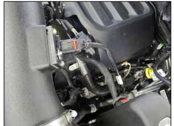
18. Reconnect the mass air sensor electrical connection.
