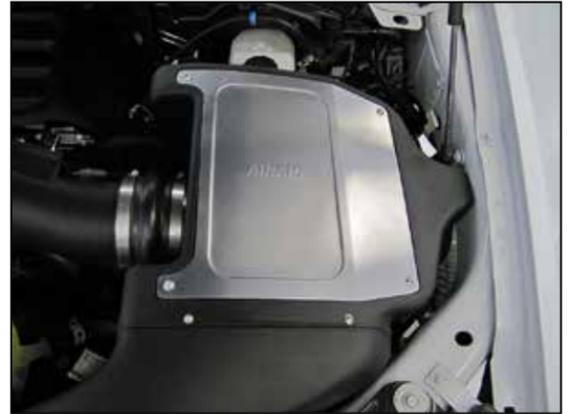
17. Install the AIRAID® air filter onto the adapter and secure with the provided hose clamp and then install the air filter housing lid and secure with the provided hardware.
