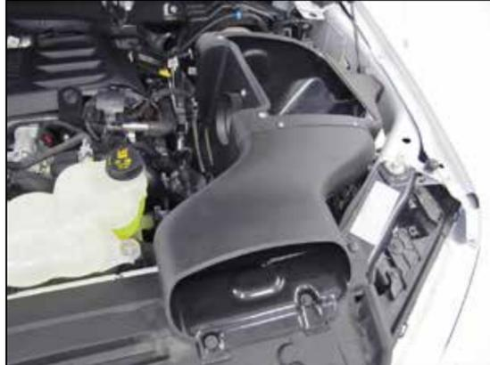
11. Install the AIRAID® air filter housing assembly into the vehicle and secure with the provided hardware.
