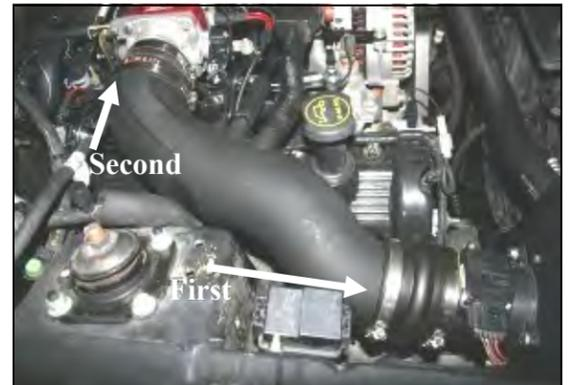
**12.** Install the Airaid Intake Tube into the hump hose first, and then onto the throttlebody. Adjust for fit, and then tighten the two remaining hose clamps. Reconnect the crankcase breather hose to the 5/8" hose, and connect the idle bypass hose to the 3/4" barbed fitting. Now reinstall the MAF sensor onto the MAF housing using the factory screws.
