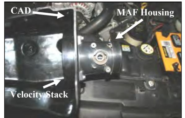
6. Mount the factory MAF housing to the Airaid Cool Air Dam (#6) using four 6mmx25mm bolts (#8), four lock washers (#10), two MAF gaskets (#12), and one velocity stack (#3). Refer to the line drawing at the top of this page for the proper sequence of how to install the parts.
