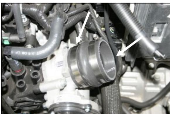
**7.** Install the supplied hump hose (#6), and two #44 hose clamps (#16) onto the throttlebody as shown. Tighten only the clamp on the throttlebody.
