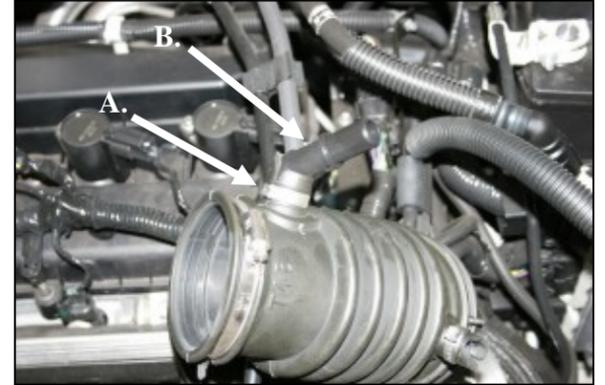
**3.** Remove the factory flexible intake tube from the vehicle. Remove the Oetiker clamp, and then remove the large plastic elbow from the flexible intake tube. It will be reused in step #12.
