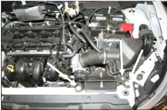
**1. Disconnect the negative battery cable!** Remove the three bolts that secure the intake scoop to the radiator support. The two long bolts will be reused in step #14.
