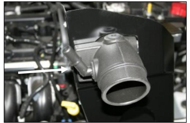
12. Insert the factory elbow removed in step #3 into the large grommet on the side of the intake tube as shown. *A drop or two of dish soap or something similar will help make the elbow slide thru the grommet easier.*
