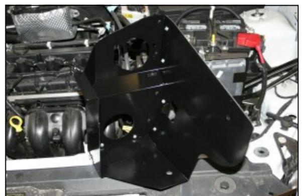
**9. Auto Transmission vehicle only:** Assemble the two Cool Air Dam panels (#3 & #4) using 7 screws (#8), washers (#9), and nuts (#10) as shown. Make sure that the bent flanges where the panels screw together, are on the outside of the box. **Note: Use panel #3 with tag marked "AUTO".**
