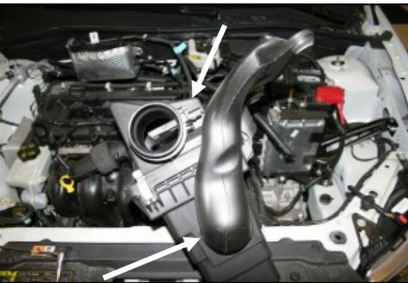
**5.** Remove the scoop from the factory airbox. Next, using the supplied #20 Torx bit, remove the Mass Air Flow sensor from the airbox lid. These parts will be re-installed in steps #10 & 13.
