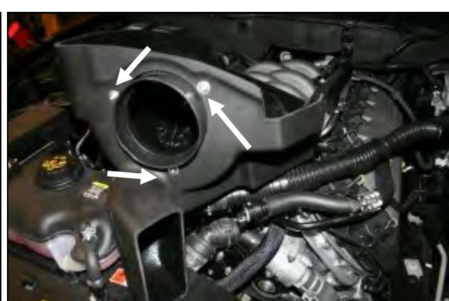
4. Install the Grommets and Fittings into the Airaid intake tube. A) All models will require the use of the 5/8" Fitting and the 5/8" Grommet. B) Automatic transmission equipped vehicles will also use the 3/8" Fitting and 3/8" Grommet. Manual transmission vehicles will not need the 3/8" components and will use the Blind Grommet.
