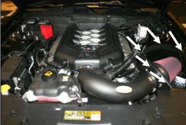
14. Install the Weather Strip (#7) onto the CAB with the contoured edge going away from the filter. Start at the front of the vehicle and work your way back. Replace the engine cover.
