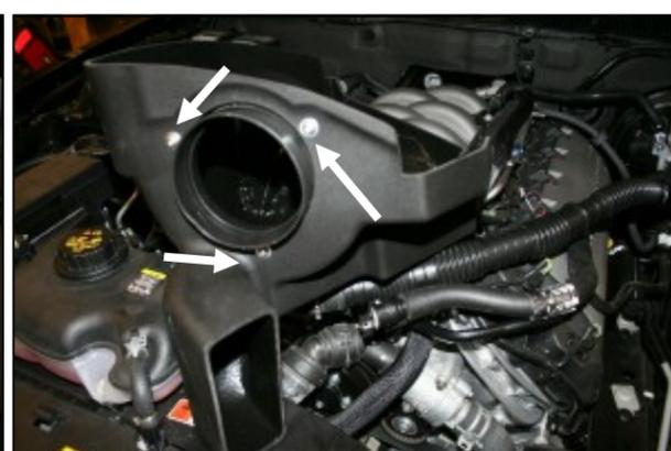
6. Install the filter adapter (#6) using three 1/4-20 button head bolts (#8), and flat washers (#9) into the Airaid Cool Air Box (CAB) (#3) as shown.
