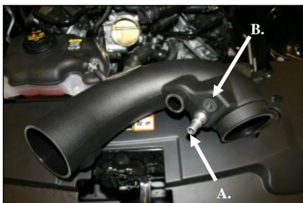
4. Install the Grommets and Fittings into the Airaid intake tube (#2). A) All models will require the use of the 5/8" Fitting (#17) and the 5/8" Grommet (#19). B) Automatic transmission equipped vehicles will also use the 3/8" Fitting (#17) and 3/8" Grommet (#20). Manual transmission vehicles will not need the 3/8" components and will use the Blind Grommet (#21).
