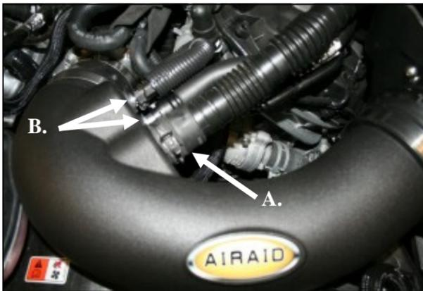
11. Install the Airaid Intake Tube into the couplers, and tighten all Hose clamps. **A)** Reconnect the Resonator tube to the Airaid Intake using the OEM clamp. **B)** Reconnect the breather line/lines to the Aluminum Fittings depending on your application. Apply the Airaid decal onto the Tube as shown.
