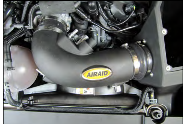
15. Insert the Intake Tube into the Hump Hose and Reducer then tighten all 4 Intake Clamps. Apply the Airaid Decal onto the Tube as shown.
