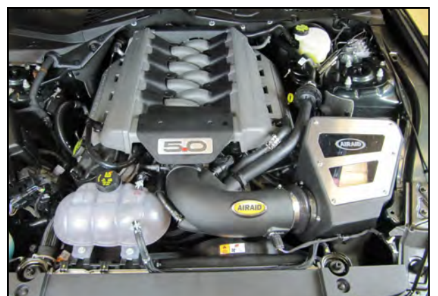
21. Double check your work. Make sure all clamps, hoses, bolts, and screws are tight. Double check the hood clearance. Reconnect the negative battery cable and reinstall the cover.
