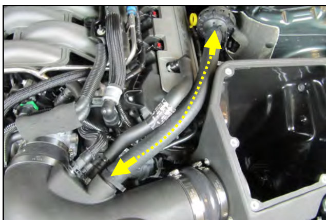
17. Connect the resonator to the Intake Tube as shown using the supplied 1" Hose and the Speed clamps on both ends.
