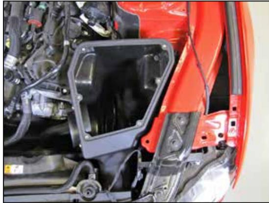
15. Install the AIRAID® air filter assembly into the vehicle and secure with the provided hardware.
