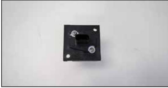
13. Remove the mass air sensor from the factory air filter housing and then install it into the provided adapter along with the provided gasket.
