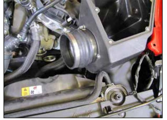
17. Install the provided hump coupler onto the filter adapter and secure with the provided hose clamp.
