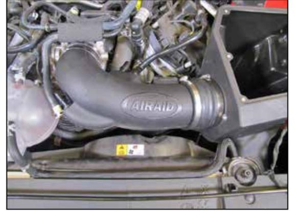
18. Install the AIRAID® intake tube into the coupler at the filter adapter and then into the coupler at the throttle body, adjust the tube for best fit and then secure with the provided hose clamps.
