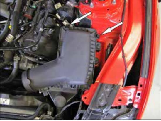
8. Release the two clips that secure the upper air filter housing and remove the upper housing from the vehicle.
