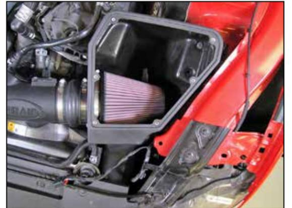
20. Install the AIRAID® air filter onto the filter adapter and secure with the provided hose clamp.
