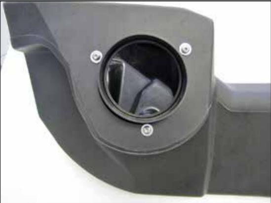
10. Install the provided filter adapter into the AIRAID® air filter housing and secure with the provided hardware.
