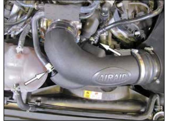
19. Connect the EVAP and crankcase vent lines to the fittings installed into the AIRAID® intake tube.
