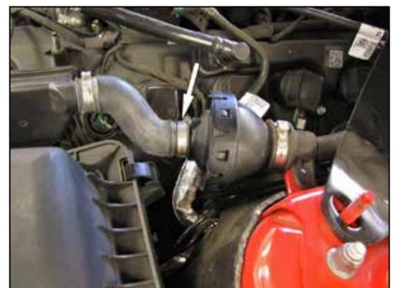
6. Release the clamp that secures the sound tube to the sound drum and then disconnect the sound tube from the drum. Remove the factory intake tube assembly from the vehicle.
