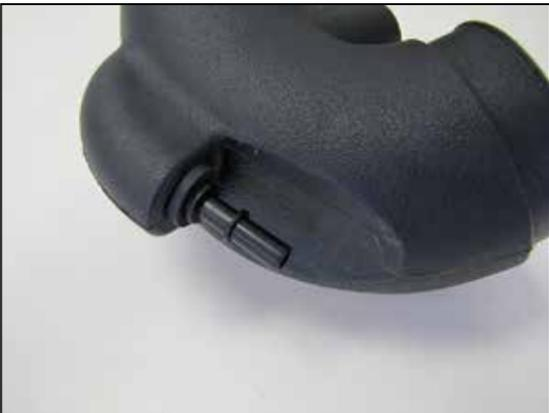
11. Install the small quick disconnect fitting into the AIRAID® intake tube using the provided grommet.
