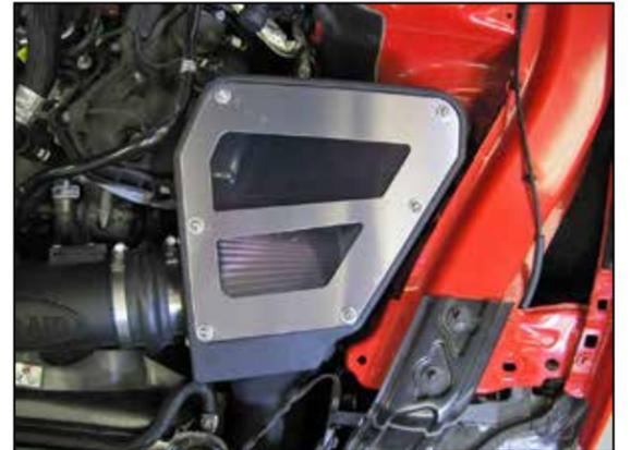
21. Install the clear and aluminum lids onto the air filter housing and secure with the provided hardware.
