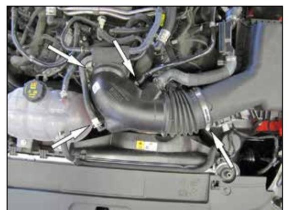
5. Disconnect the two vent lines attached to the factory intake tube, loosen the hose clamps that secure the intake tube to the throttle body and air filter housing.
