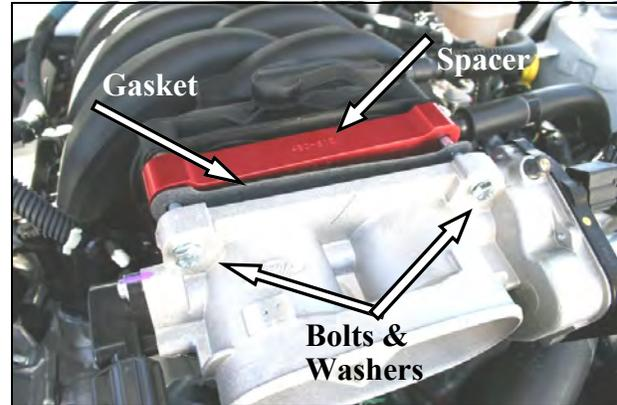
4. Install two bolts (#2), and washers (#3) thru the throttle body, thru the gasket (#4), thru the AIRAID Spacer (#1), and into the intake manifold as shown. **Use caution to retain the factory o-ring gasket on the plastic intake manifold.**
