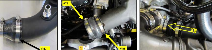
9. Slide the Reducer and Clamps onto the turbo side of the Intake Tube as shown. Leave the clamps loose for now.
