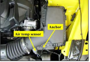
2. Loosen the clamp on the intake tube and slide it off of the airbox. Gently pry the harness anchor out of the airbox and disconnect the air temp sensor.
