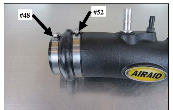
6. Slide the Hump Hose, one #48 Clamp, and one #52 Clamp onto the Intake Tube as shown. Do not tighten the Clamps at this time.
