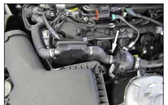
6. Release the one-time use clamp that secures the sound tube to the drum and then disconnect and remove the sound tube from the vehicle.
