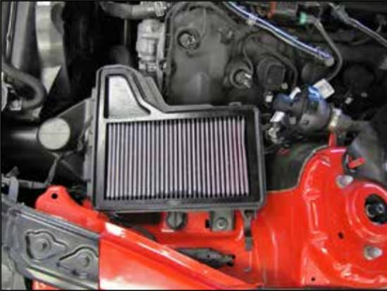
8. Release the clips that secure the upper air filter housing and then remove the factory air filter. Install the AIRAID® replacement air filter and resecure the upper housing with the factory clips.
