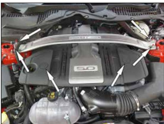
2. Remove the four nuts that secure the strut brace and then remove the strut brace from the vehicle. Pop up the two-round bolt covers.
