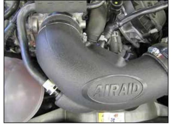
12. Install the AIRAID® intake tube assembly into the coupler hoses, adjust for best fit and then secure with the provided hose clamps. Connect the factory vent lines to the fittings installed into the intake tube.
