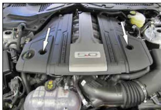
3. Remove the two nuts that secure the decorative engine cover and remove the cover from the engine.
