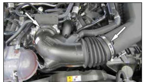
5. Loosen the hose clamps that secure the intake tube to the air filter housing and throttle body and then remove the intake tube from the vehicle.
