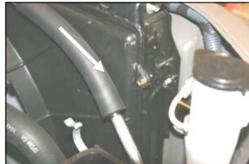
**5. Remove fan shroud bolt on passenger side of radiator, save for later use.**
