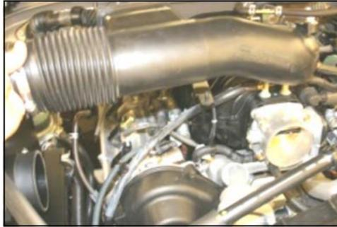
14. Remove the factory intake tube.
