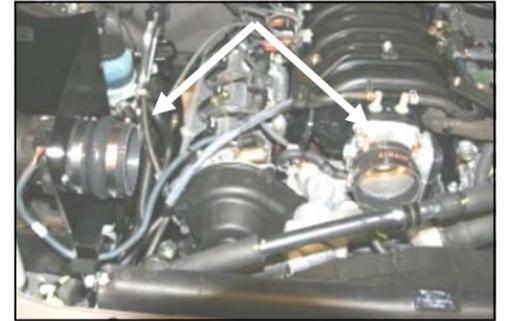
15. Install the hump hose (#7) on the MAF adapter (#4) with two hose clamps (#11). Install the reducer (#6), small end first, onto the throttle body with two hose clamps (#10). Leave the clamps loose for now.
