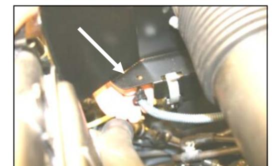
**9. Slip hose mount (#21) over MAF wire harness, and into hole in bottom of CAD. This will keep the harness from chafing.**
