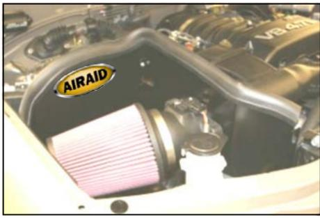
10. Install the Airaid Premium Filter (#1) on the MAF adapter. Next install the weather strip (#9) on the CAD as shown. Start at the front, next to the radiator, and work your way towards the back.
