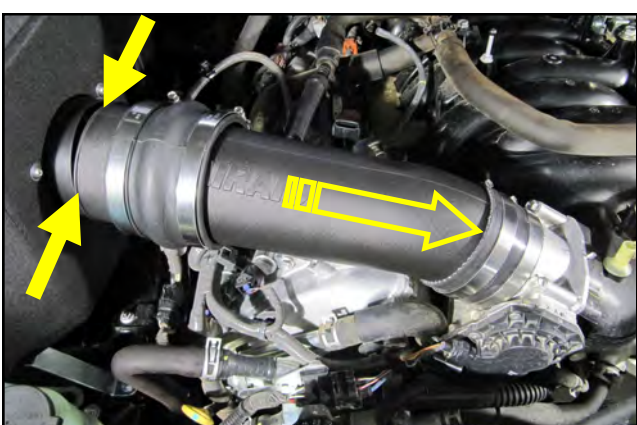
19. Insert the Intake tube into the Reducer and align Hump Hose with the Filter adapter in the Airbox.
