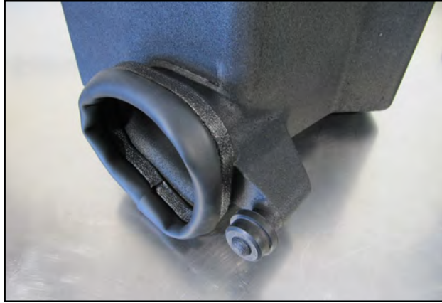
8. Install the Edge Trim onto the Airaid airbox inlet. Trim excess if necessary. Hint: Relaxing the crimp on the Edge Trim with screwdriver or similar will ease the installation.
