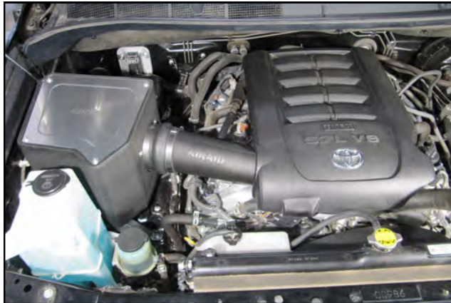
26. Slowly lower the hood to test clearances. Make sure all clamps, hoses, bolts, and screws are tight. Double check the hood clearance. Reconnect the Negative battery terminal.
