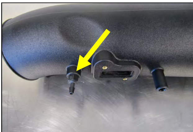
14. Insert the NPT Barbed Fitting into the Airaid Intake Tube as shown.
