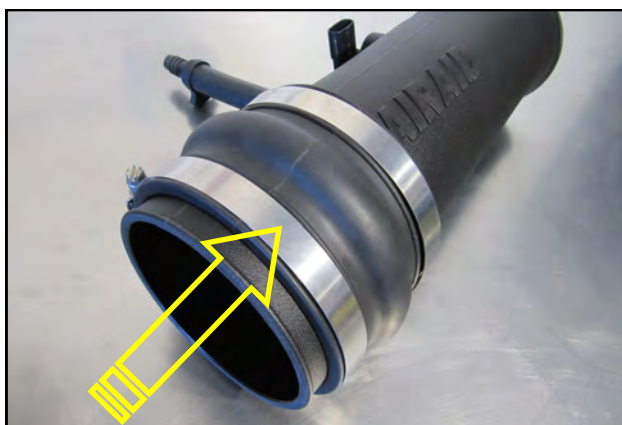
17. Slide the Hump Hose with the two 72 Clamps all the way onto the Intake tube as shown.
