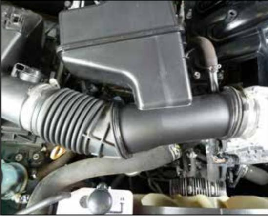
4. Disconnect the vent line attached to the factory intake tube and then loosen the two hose clamps that secure the tube. Remove the intake tube from the vehicle.
