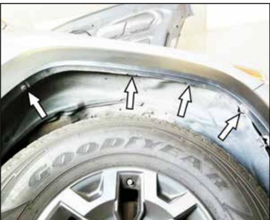
8. On vehicles equipped with fender flares, remove the four bolts that secure the flare to the fender.
