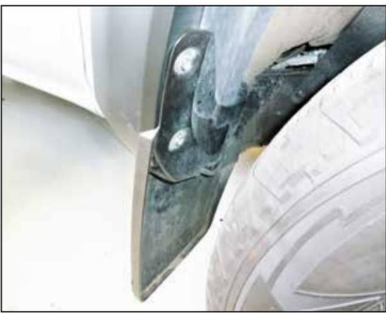
7. Remove the mud flap if equipped.
