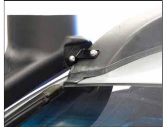
27. Install the upper mounting bracket and secure with the provided hardware.
