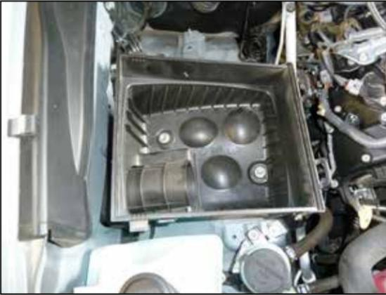
31. Reinstall the lower air filter housing and secure with the factory hardware. Secure the snorkel duct to the air filter housing with the provided hose clamp. **NOTE: It may be necessary to move the washer bottle to gain access and tighten the hose clamp.**
