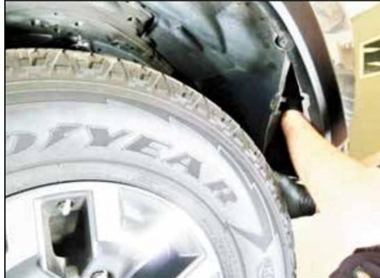
10. On vehicles equipped with fender flares, Pull the inner fender back and reach in to release the three clips that secure the front side of the fender flare. Pull the fender flare off the fender. **NOTE: the flare is held on with two different style clips that may be destroyed while removing the flare. New clips are included for reassembly.**
