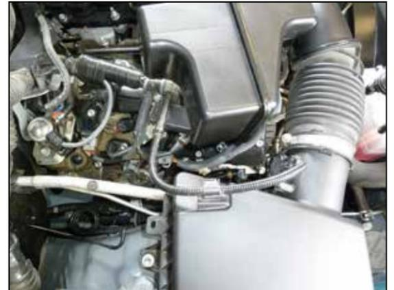
34. Reconnect the mass air sensor electrical connections and secure the wiring harness.
