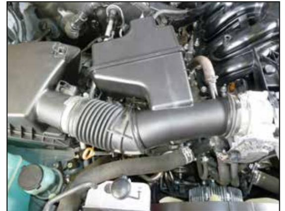
33. Reinstall the intake tube and secure with the factory hose clamps. Reconnect the vent lines.
