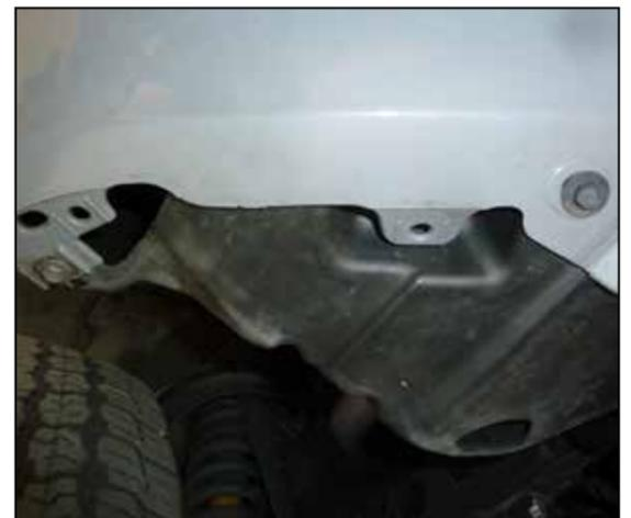
29. Replace the two inner fender retaining clips with the clips provided and then reinstall the two factory screws.
