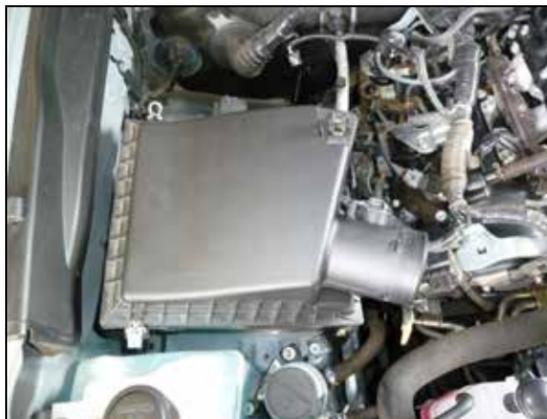
32. Install the air filter and upper housing.
