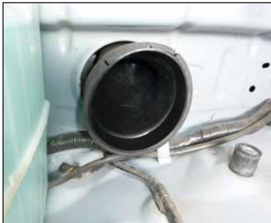
31D. Install the flexible spacer into the flexible duct as shown and then the AIRAID air filter housing can be installed.
