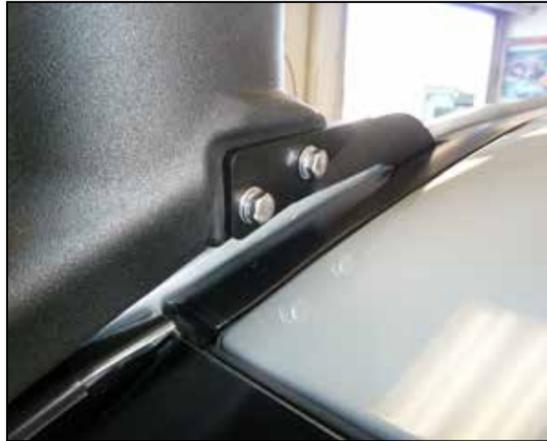
22. On vehicles without a factory TOYOTA roof rack, install the snorkel onto the fender and secure it to the top mounting bracket with the hardware provided.
