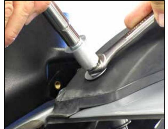
26. Using a 9/16" wrench to hold the nut and a 10mm socket and ratchet to tighten the bolt while applying downward pressure on the bolt. This compresses the Rivnut and grips the plastic of the roof rack. Tightening force will be high initially and then lessen until the Rivnut is set. Force will ramp up again once set, do not over tighten.
