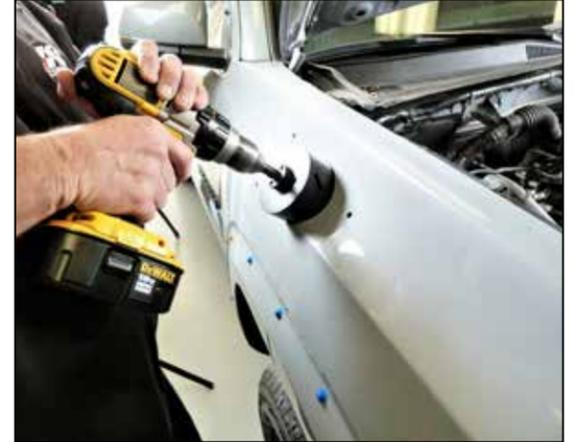
14. Drill three 1/2" holes for the snorkel mounting location and using a 4" hole saw, drill the 4" hole for the air duct. **NOTE: the 4" hole will be drilled through different angled surfaces, use caution while drilling to not distort the remaining sheet metal.**
