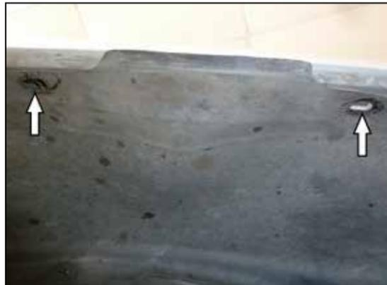
11. Remove the screws from the top two black plastic clips that secure the top of the inner fender and then remove the two clips. **NOTE: The easiest way to remove these clips is to cut the tops off with side cutters and then push the remaining parts through the fender. New clips are provided.**
