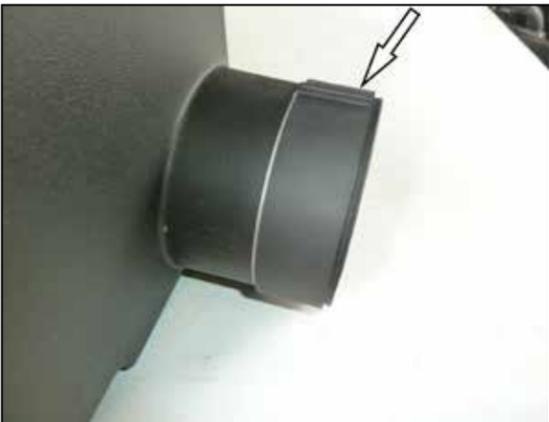
31A. if using an AIRAID intake kit, install the provided flexible spacer onto the AIRAID filter housing inlet as shown. Using a marker, draw a line around the inlet using the spacer as a guide.
