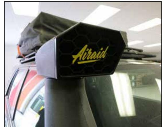
28. Install the snorkel scoop onto the snorkel and secure with the provided hose clamp.
