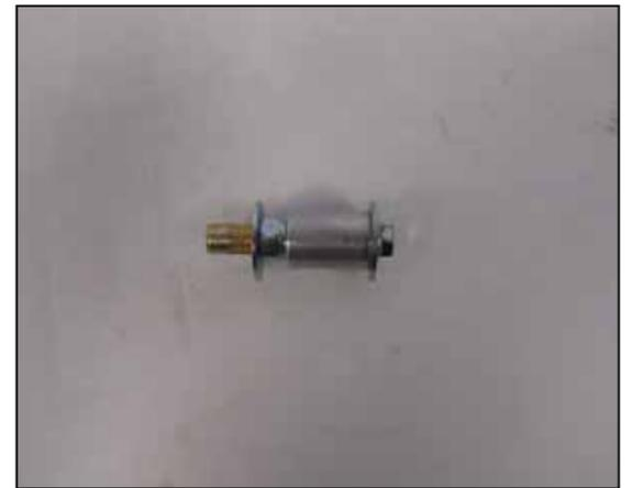
25. If a Rivnut setting tool is not available, assemble the provided hardware as shown to install the Rivnut. **NOTE: The nut passes over the threads of the bolt, it does not thread on.**
