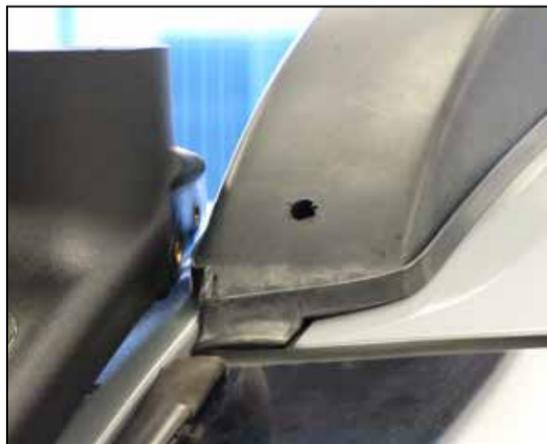
24. Drill a 1/8" id pilot hole into the marked location on the roof rack and then drill a 25/64" id hole.
