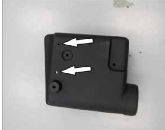
31C. Drill two 3/8" id holes into the bottom of the AIRAID air filter housing for water drainage.
