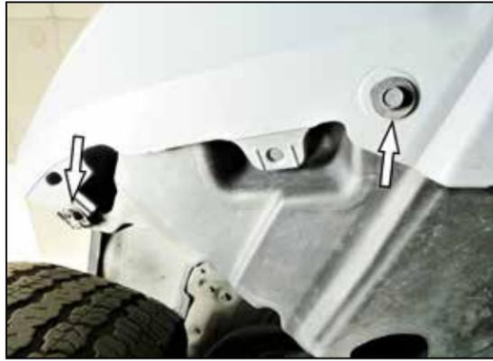
9. Remove the two bolts that secure the inner fender to the bottom of the front bumper cover.
