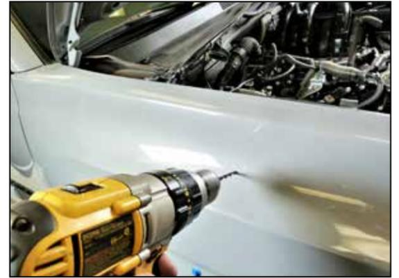
13. Drill a 1/8" pilot hole in all four locations to be drilled.
