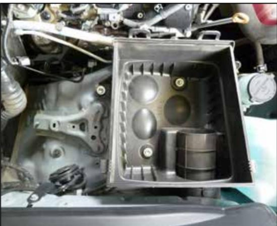
6. Remove the three bolts that secure the lower air filter housing and then remove the housing from the vehicle.
