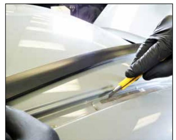
17. Using a knife, slice the sealing tape to allow access to the inserted nuts. **NOTE: Do not remove the tape, slicing the tape will allow the bolt to pass through.**
