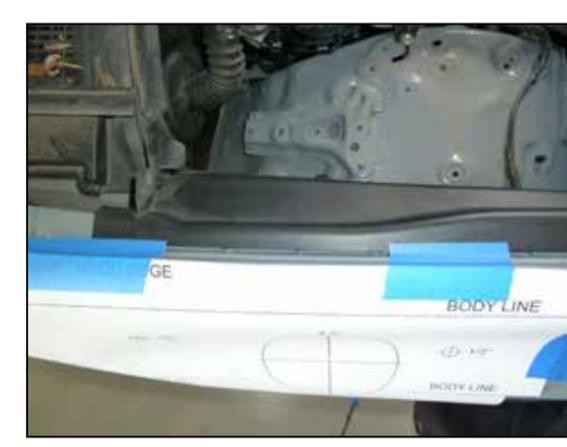
12. Cut the hole template provided and tape together. Tape the assembled template to the front fender as shown. Using the template guide, mark the four locations in the fender that will be drilled with a center punch or similar device. **NOTE: The fender sheet metal is thin, light tapping is all that is needed to mark the hole location.**
