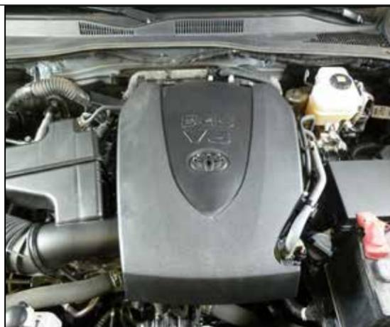
2. Lift up the engine cover and remove it from the vehicle.
