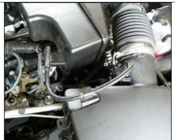
3. Disconnect the mass air sensor electrical connection and unhook the wiring harness from the air filter housing.
