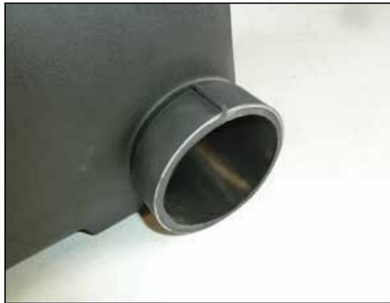
31B. Cut the inlet of the housing at the marked line.
