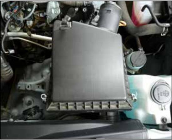
5. Release the clips securing the air filter housing lid and then remove the lid and air filter.
