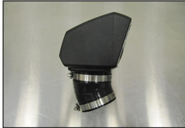
13. Install the Silicone Elbow (#6) and two #48 clamps onto the Inlet a shown. Leave the Hose Clamps loose for now.
