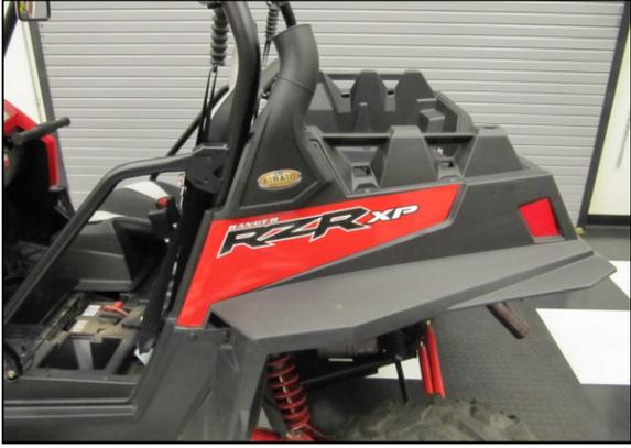
9. Re install the fender onto the vehicle, reusing the nine fasteners from step 2. Install the Airaid decal as shown.
