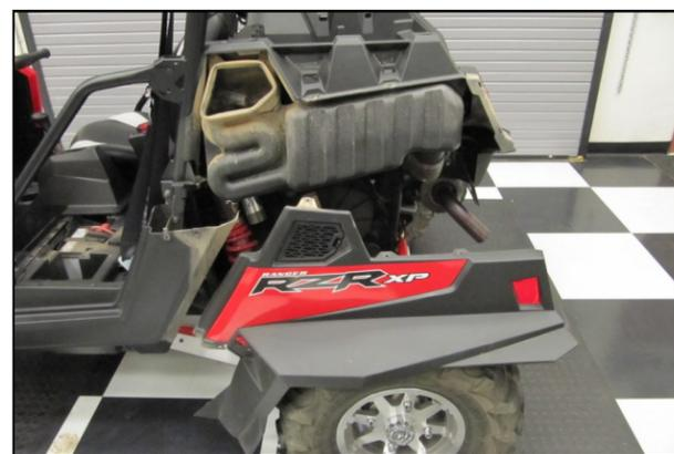
**2.** Starting on the Drivers side first, remove the nine T-27 Torx head screws holding the fender in place. Remove the fender and place it on a work bench.
