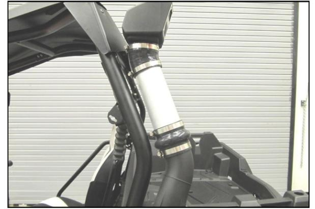
14. Install the Snorkel Inlet and elbow onto the Intake tube. Align the assembly into the desired position and tighten all of the Clamps.
