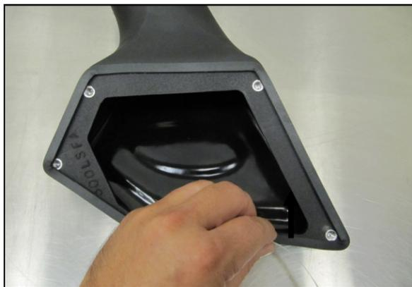
**7.** Prepare the mating surface of the Fender Adapter (#1) for the Foam Gasket Tape (#13) by cleaning with a prep solvent. Apply the gasket tape along the outside edge of the Fender Adapter as shown, avoiding the bolt holes.
