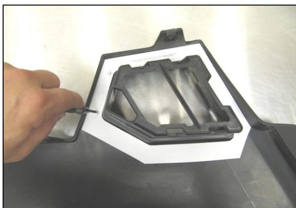
**4.** Cut out the paper Template. Align it with the edges of inner fender, and punch the four pilot holes.
