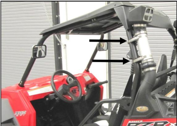
15. Secure the snorkel assembly to the roll cage using the Tube Mounts (#8) and #68 Clamps (#11).
