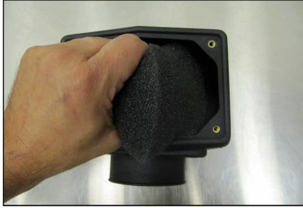
10. Insert the Foam Pre Filter (#5) into the Snorkel Inlet (#3).
