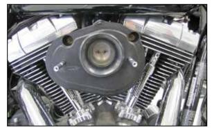
10. Install the filter base plate onto the throttle body using the factory breather bolts and the throttle bolts installed during step #7. Alternate the tightening sequence between all five bolts until the base plate is completely tight.
