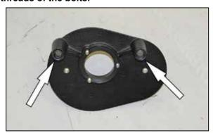
9. Install the two provided O-rings onto the filter base plate as shown.
