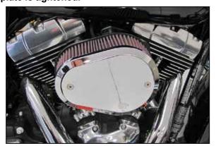
11. Set the top plate onto the air filter and then install the filter assembly onto the vehicle and secure with the provide hardware.
