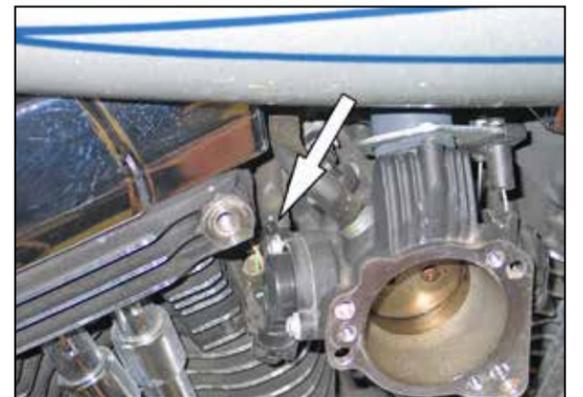
6. Using the provided tie wrap, secure the wiring pig tail to the throttle body wiring harness. **NOTE: On non-US models, a by-pass module (sold separately) will need to be installed onto the pigtail to eliminate an engine management light from turning on. (non-US models only)**
