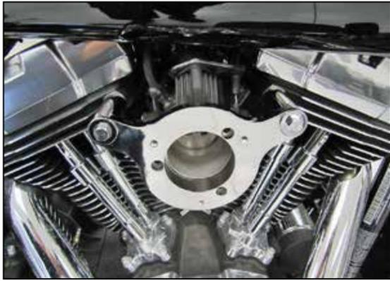
8. Install the K&N® crankcase breather plate along with the two remaining o-rings, mounting bolts (with one drop of thread locker) and the throttle body gasket as shown.
