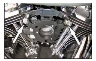
6. Install the K&N® adapter onto the engine and throttle body using the provided breather bolt. NOTE: Do not completely tighten the breather bolts at this time. Take care while installing the adapter so that the "O" rings do not get pinched.
