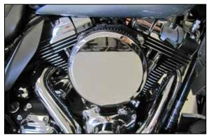
13. Install the K&N® air filter and front plate onto the back plate and secure with the provided hardware. NOTE: It may be helpful to use a small screwdriver to position the filter into the grooves of the front and back plate while tightening the hardware.
