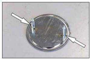
12. Install the provided mounting studs onto the front plate with the provided lock washers.
