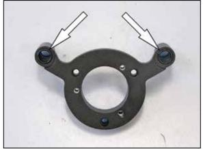
5. Install the four provided "O" rings into the K&N® base plate as shown.
