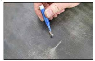
10. Apply one drop of the provided thread locker to the provided filter back plate mounting bolts.
