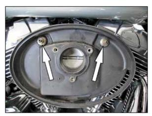
4. Remove the two breather bolts and then remove the inner air filter base.
