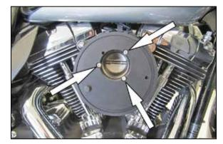
11. Install the filter back plate and gasket onto the adapter and secure with the provided bolts.
