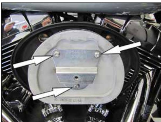
3. Remove the three bolts securing the air filter, then disconnect the crank case breather hoses and remove the air filter.
