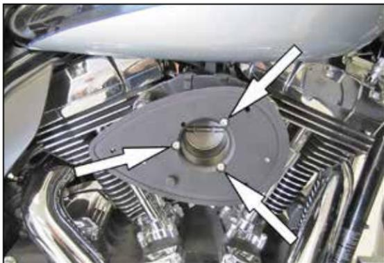
13. Install the filter back plate and gasket onto the adapter and secure with the provided bolts.
