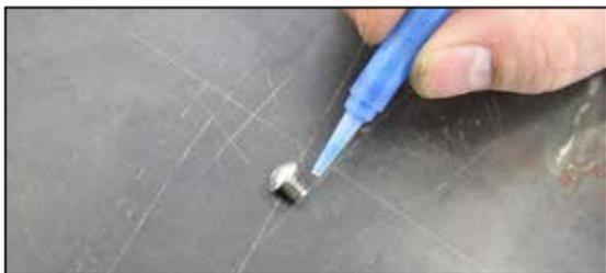
10. Apply one drop of the provided thread locker to the two provided filter back plate bolts.
