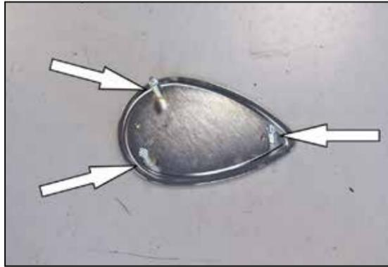
14. Install the provided mounting studs onto the front plate with the provided lock washers.
