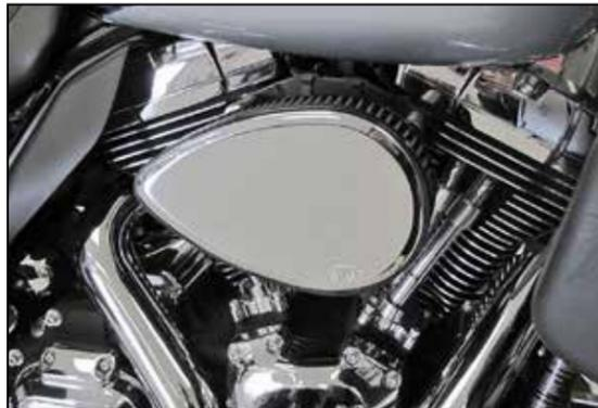
15. Install the K&N® air filter and front plate onto the back plate and secure with the provided hardware.
