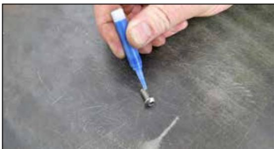
12. Apply one drop of thread locker to the back plate mounting bolts.
