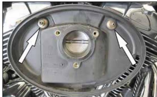
4. Remove the two breather bolts and then remove the inner air filter base.
