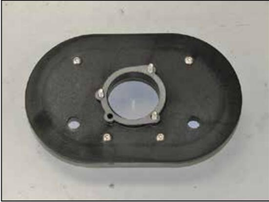
9. Install the provided throttle body gasket onto the back plate as shown.
