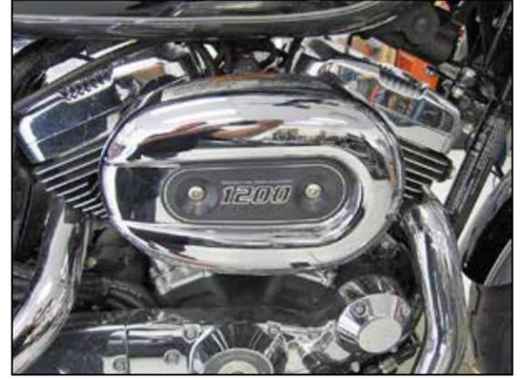
13. Remove the rubber seal from the factory air filter bonnet and then install the bonnet onto the air filter and secure with the factory hardware. Reconnect the negative battery cable.
