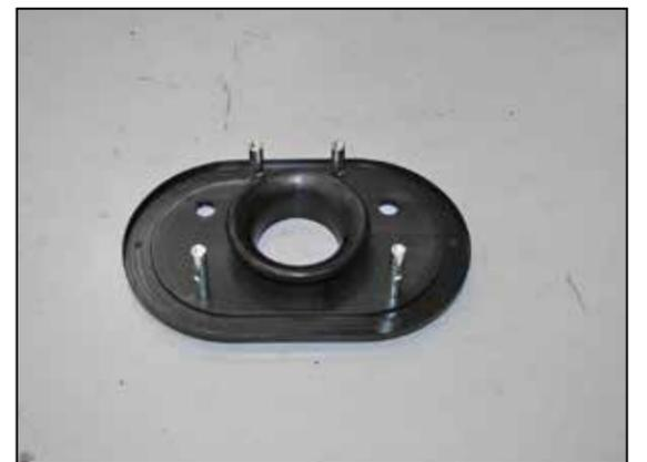
7. Install the provided venturi into the K&N® back plate as shown.
