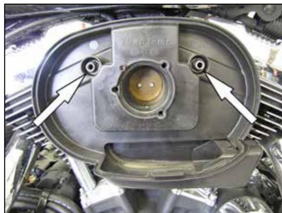
4. Remove the two stock breather bolts shown and then remove the factory filter back plate.
