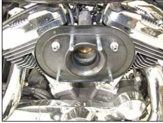
11. Install the back plate assembly onto the throttle body and then secure with the two factory breather bolts and the three throttle body bolts.
