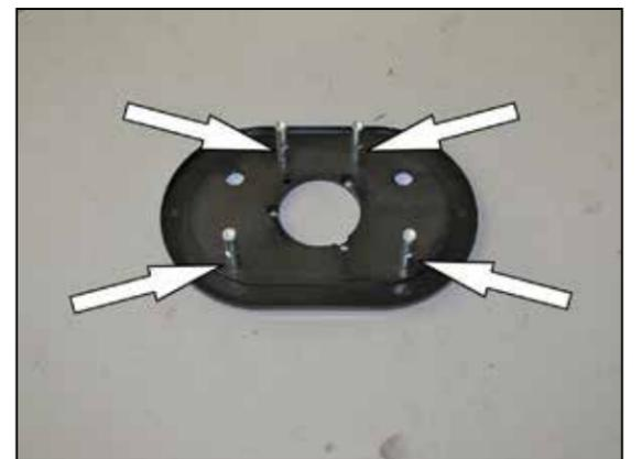
6. Install the four provided stand-offs onto the K&N® back plate using the provided hardware. Be sure to place one drop of the supplied thread locker onto the bolts before assembly.
