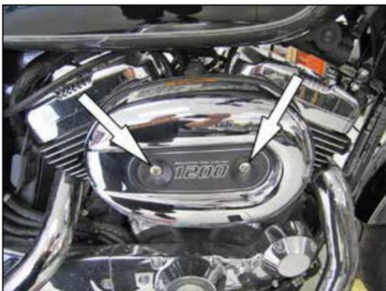
2. Remove the two bolts that secure the factory filter cover and then remove the filter cover.
