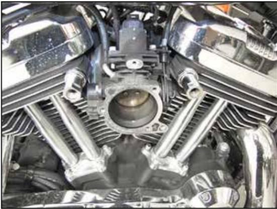
10. Place one drop of thread locker onto the threads and then install the two provided breathers onto the cylinder heads as shown.
