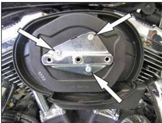
3. Remove the three bolts that secure the factory air filter and then remove the air filter.
