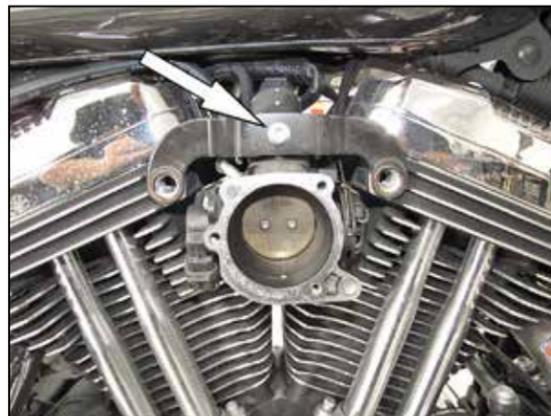
5. Remove the bolt shown securing the throttle body bracket and then remove the bracket.
