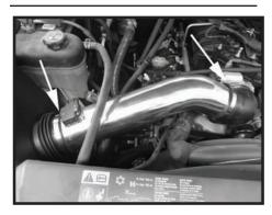
Step 17 Install the intake tube as shown and once in position tighten clamps.
