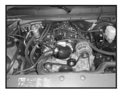
Step 14 Install the 90° boot on throttle body with the short side on the throttle body and clamp on the throttle body side to secure the boot in place. Install a second clamp but do not tighten at this time.
