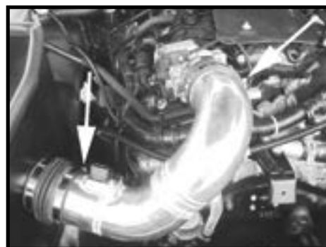
Step 15 Install the intake tube as shown and once in position tighten clamps.
