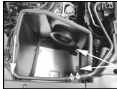
Step 13 Install the heat shield into the vehicle. Reuse the factory nuts from Step 7 and 12 to securely fasten the heat shield in place.
