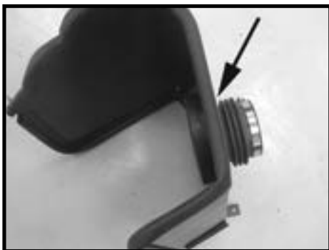
Step 11 Place the velocity stack adapter in the heat shield and install the supplied flex coupler making sure the coupler is pushed completely against the heat shield. Once the adapter and coupler are tight against the heat shield, tighten the clamp. Install a second clamp but do not tighten at this time.
