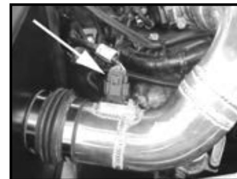
Step 16 Reconnect the MAFS wiring harness.
