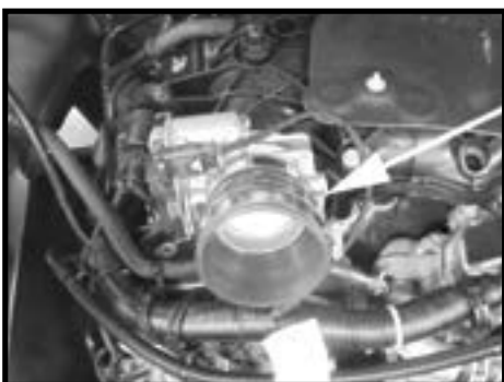
Step 14 Install the reducer coupler on the throttle body and secure the coupler in place. Install a second clamp but do not tighten at this time.
