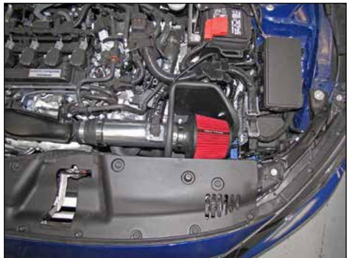
12. Reconnect the maf sensor electrical connection.
