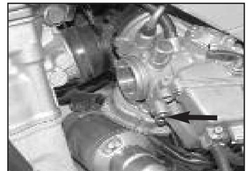
9. Locate fuel mixture screw and turn screw clockwise until lightly seated. Now turn screw counterclockwise 2-1/2 turns.
