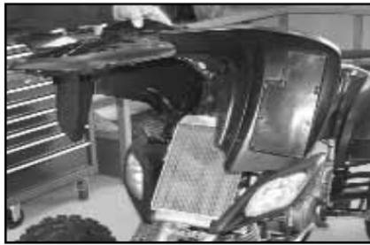
6. Remove the front fender assembly.
