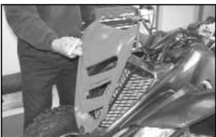
4. Remove the fasteners from the front plastic shell that sits over the radiator and remove the plastic shell.
