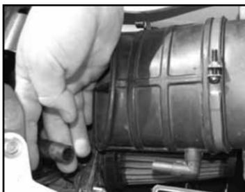
30. Disconnect the crankcase breather hose from the intake snorkel on the air box lid.
