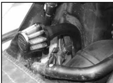
33. Install the oiled crankcase breather filter into the crankcase breather hose.
