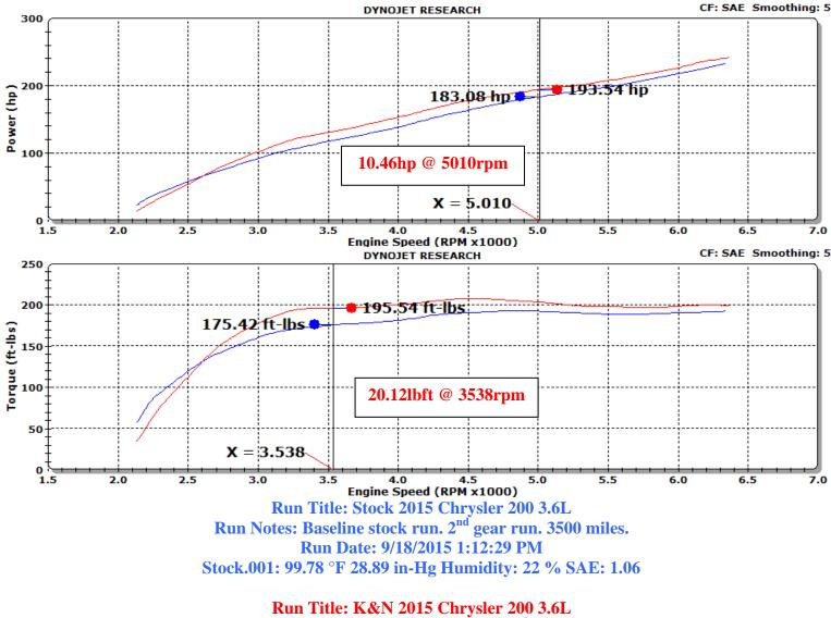
Run Title: K&N 2015 Chrysler 200 3.6L Run Notes: K&N intake kit #63-1572 installed. 2<sup>nd</sup> gear run. 3500 miles. Run Date: 9/18/2015 2:16:29 PM K&N.002: 103.00 °F 28.89 in-Hg Humidity: 17 % SAE: 1.06
