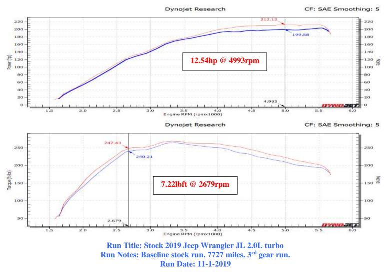
Run Title: K&N 2019 Jeep Wrangler JL 2.0L turbo Run Notes: K&N intake kit #57-1580 installed. 7727 miles. 3<sup>rd</sup> gear run. Run Date: 11-1-2019
