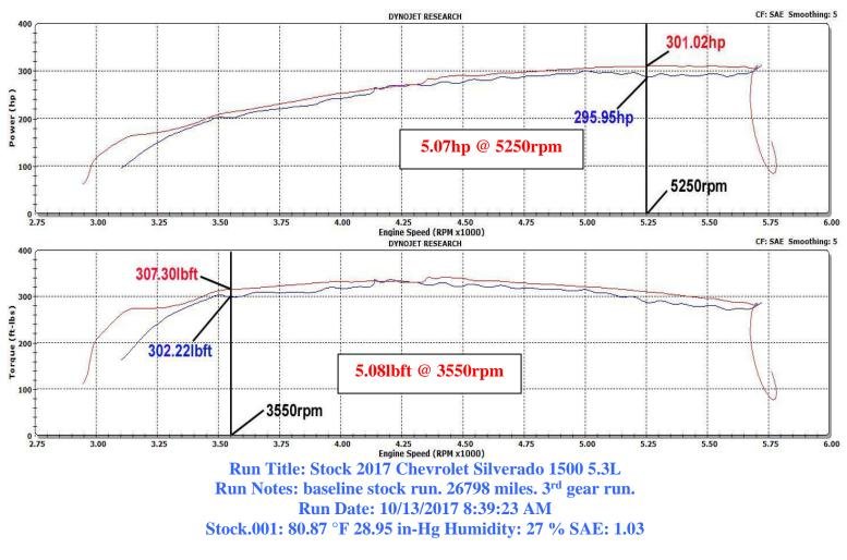
Run Title: K&N 2017 Chevrolet Silverado 1500 5.3L Run Notes: K&N intake kit #57-3098 installed. 26798 miles. 3<sup>rd</sup> gear run. Run Date: 10/13/2017 8:59:39 AM K&N.002: 82.96 °F 28.97 in-Hg Humidity: 26 % SAE: 1.03
